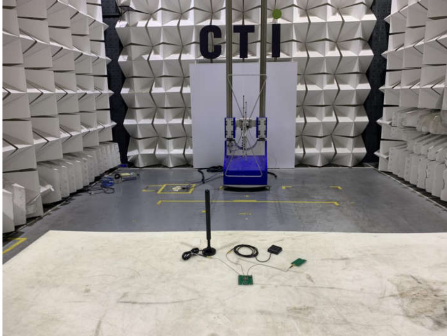
Radiated spurious emission Test Setup-1(Below 1GHz)
