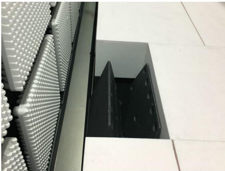
Radiated spurious emission Test Setup-5(Above 1GHz) There are absorbing materials under the ground.
