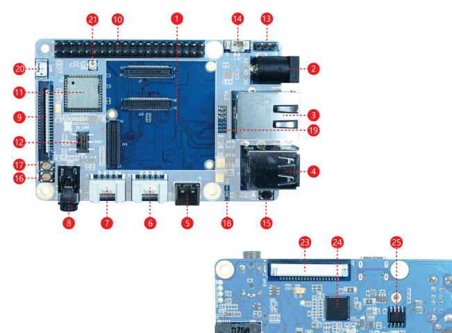
1.Seeed SoM-STM32MP157C Installation Area: If the user wants to remove the core board, slowly tilt the core board up and then remove. Never remove by hand.
