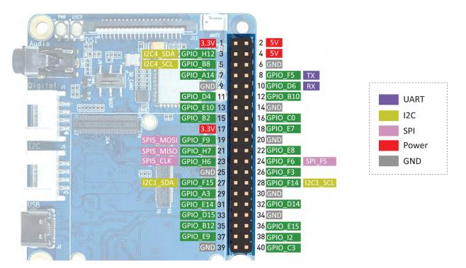
ODYSSEY - STM32MP157C's 40-pins are fully compatible with Raspberry Pi's 40-pins including GPIO, I2C, UART, SPI, I2S and PWM pins.
