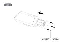
**Note:** During the installation, ensure that the waterproof washer is properly installed and the screws are locked; otherwise, water will flow into the device.
