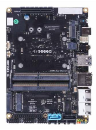
ODYSSEY X86 v2 board powered by the latest Intel® Core<sup>™</sup> 11th Gen. processor and Intel® UHD Graphics or Intel® Iris Xe Graphics, which delivers high CPU and AI performance for various applications. It has two high-speed 2.5-Gigabit Ethernet ports and supports hybrid connectivity including, BLE and WIFI. Meanwhile.
