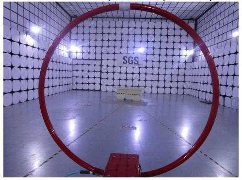
1.5 Radiated Emissions(30MHz-1GHz) Test Setup
