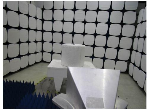
1.3 Radiated Spurious Emissions Test Setup
