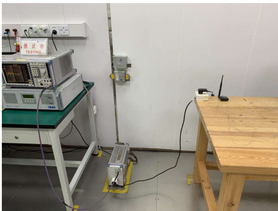
Conducted Emissions Test Setup
