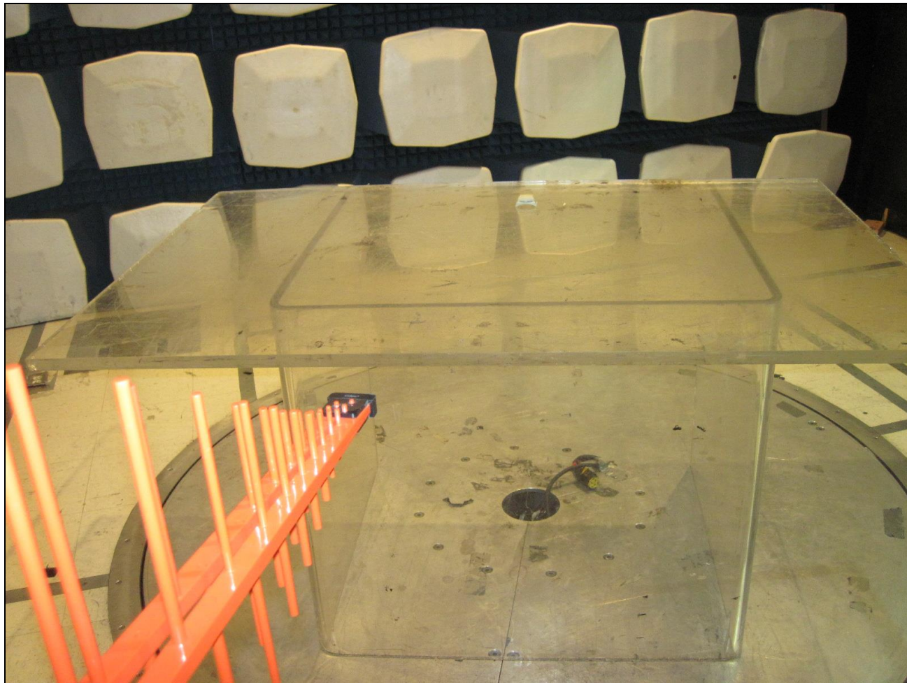
Photograph 3. Radiated Spurious Emissions, Test Setup
