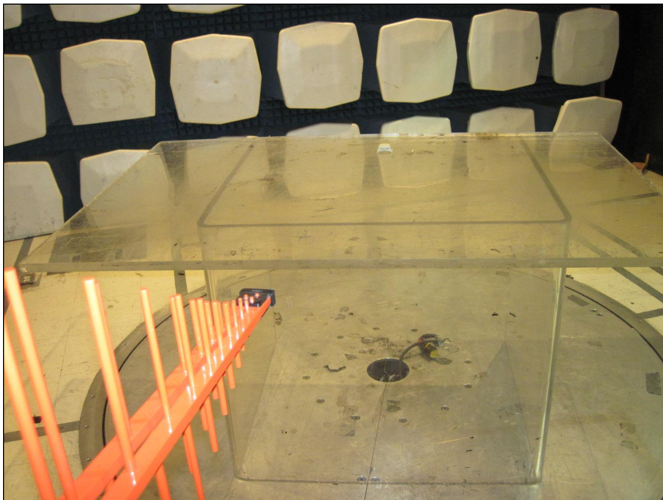
Photograph 2. RF Output Power, Test Setup
