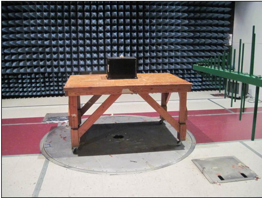
Photograph 8. Radiated Spurious Emissions, Bilog
