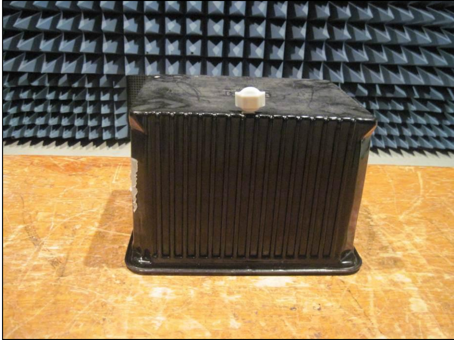
Photograph 7. Radiated Spurious Emission, Test Setup
