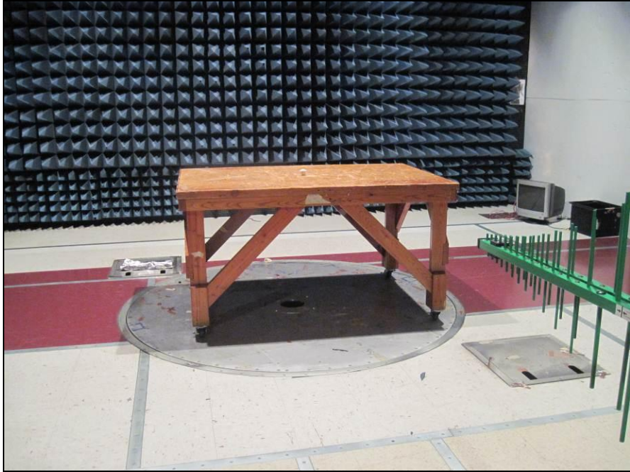
Photograph 3. Radiated Emission, Test Setup, Bilog Setup
