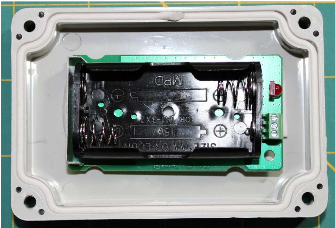
Fig 18. Close up of the Battery Compartment Left-hand side, showing the wire antenna placement.
