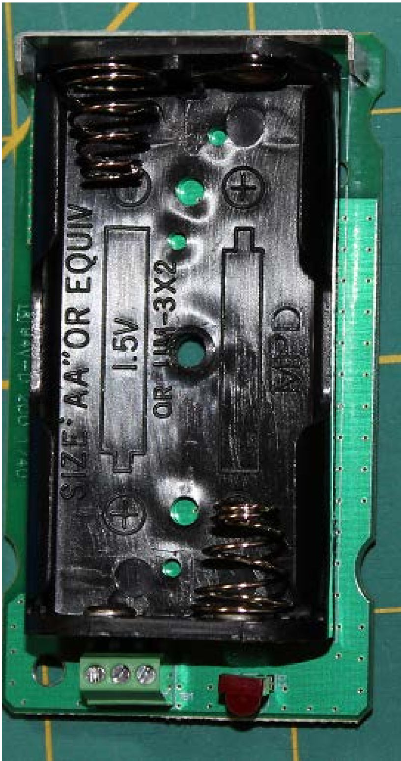
Fig .10 PCB assembly from the top showing through-hole components.
