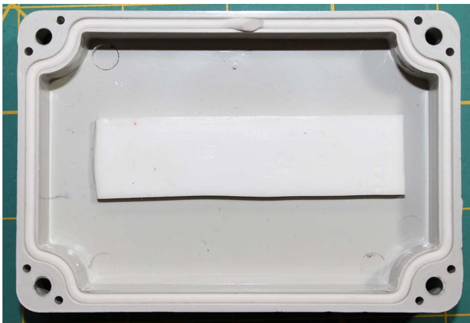
Fig 22. Inside of Top Cover, showing double sided sticky tape mounting mechanism
