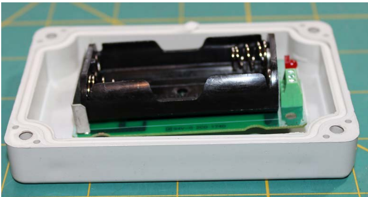
Fig 18. Close up of the Battery Compartment Left-hand side, showing the wire antenna placement.
