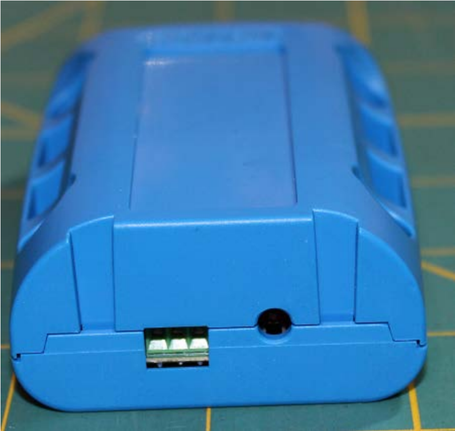
Fig. 6 Trailing edge showing the LED and terminal block for external wiring to sensors.
