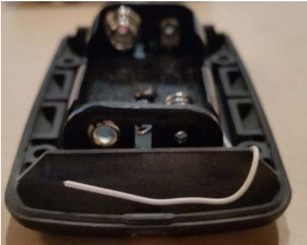
Fig. 6, Front of assembly showing antenna
