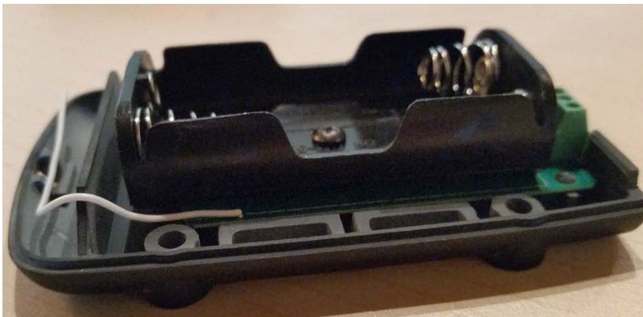
Fig 3. Close up of the Battery Compartment Left-hand side, showing the wire antenna placement.
