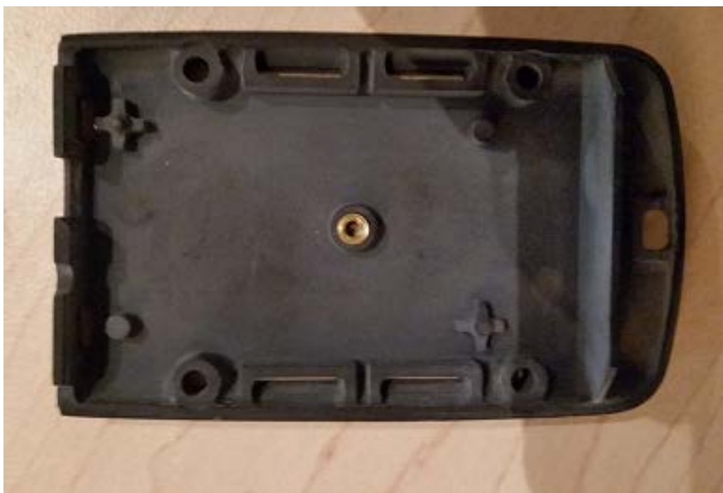
Fig 8. Bottom of enclosure with circuit board and battery compartment removed.
