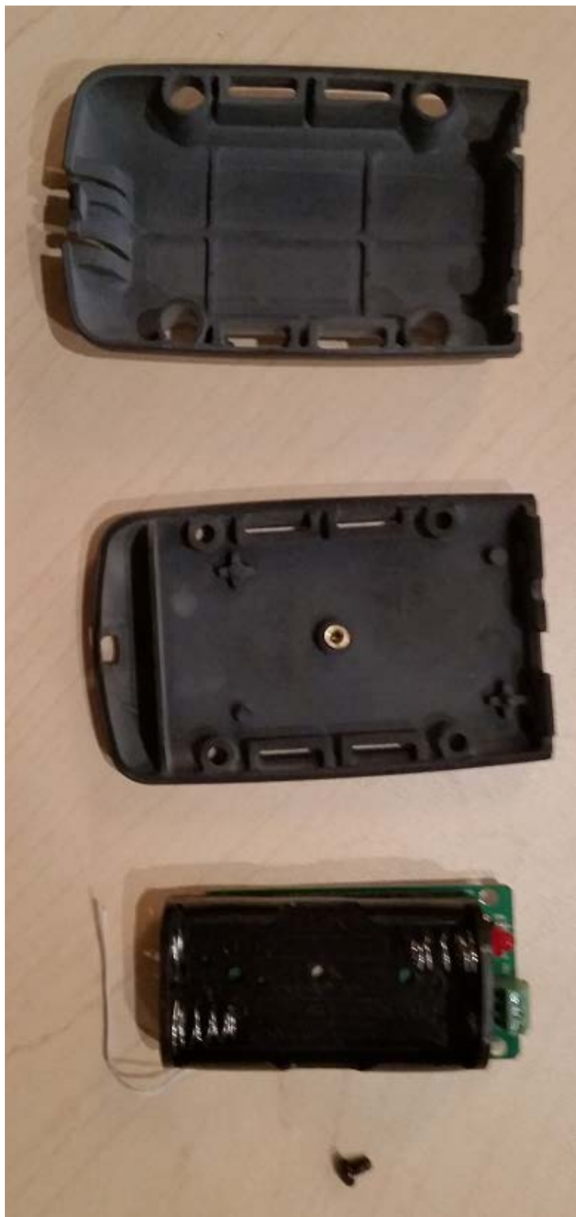
Fig. 9. All components required to assemble the remote wireless sensor.
