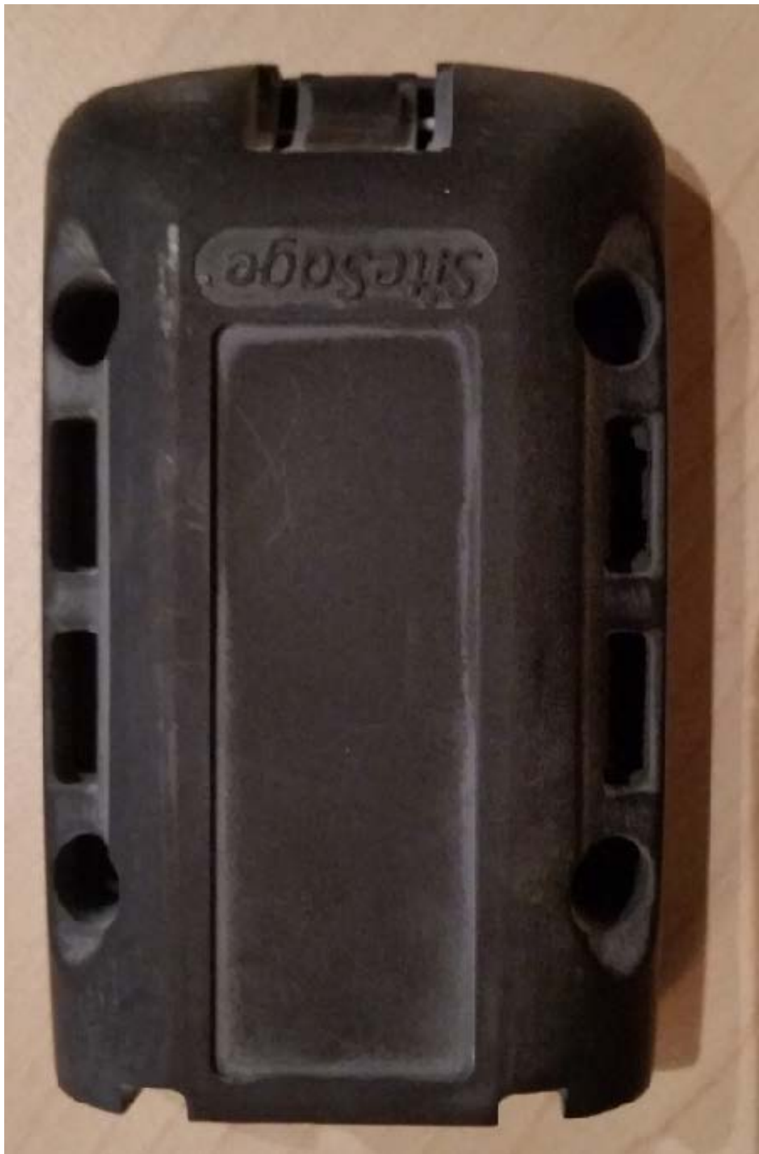
Fig 1. Top of Enclosure,. Showing battery compartment clasp at top.
