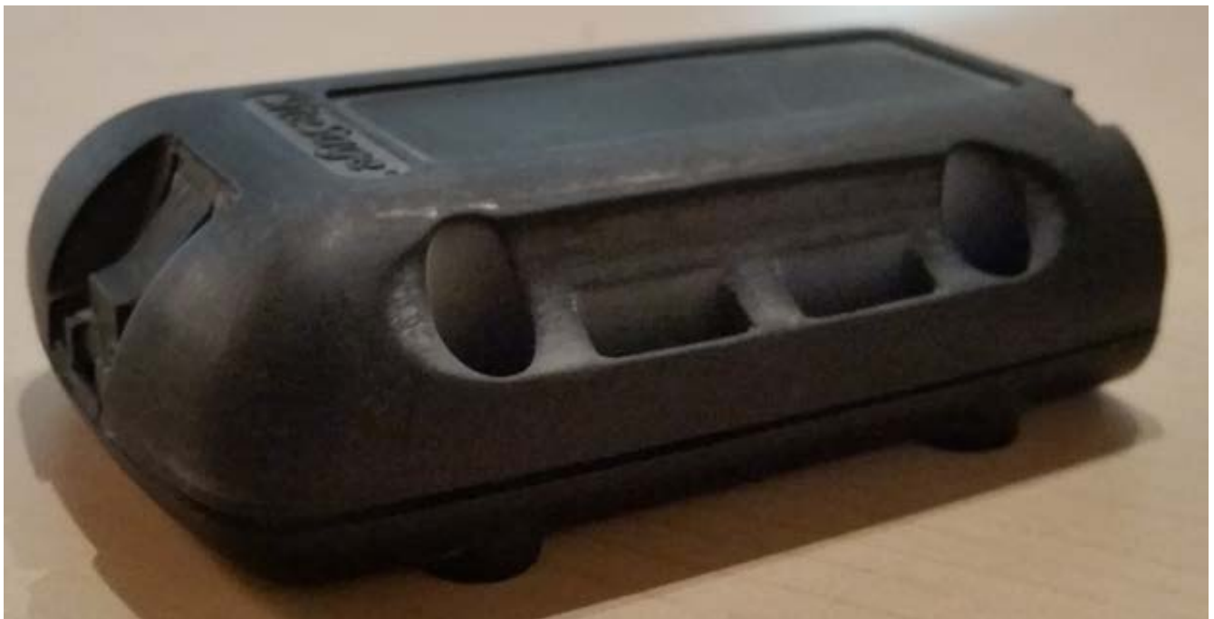
Fig 4, Left-hand side of module, battery compartment clasp showing left-hand edge.
