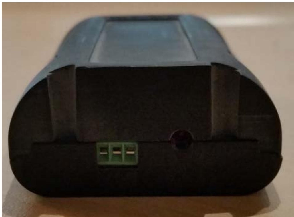
Fig. 6 Trailing edge showing the LED and terminal block for external wiring to sensors.
