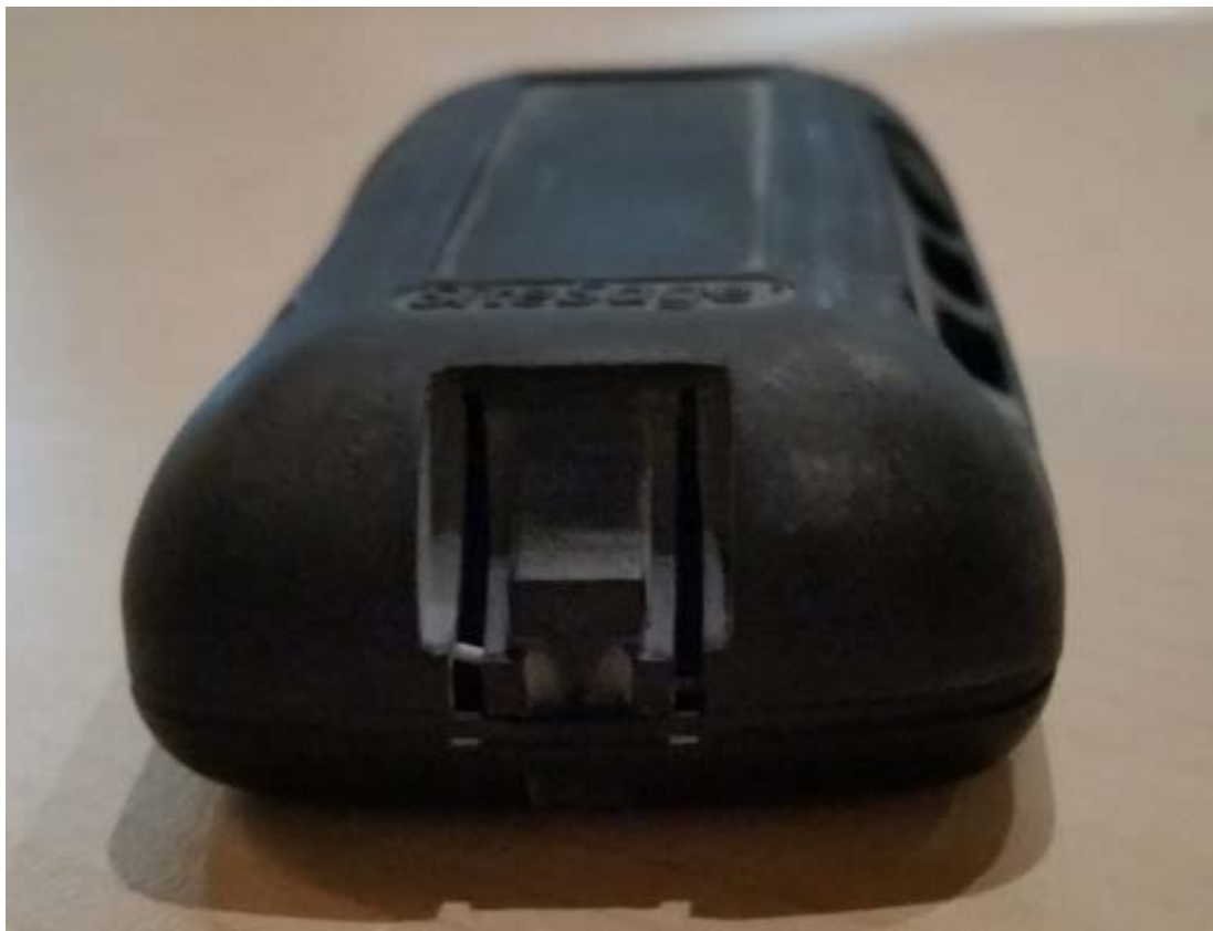
Fig.5, Leading edge showing battery compartment clasp.
