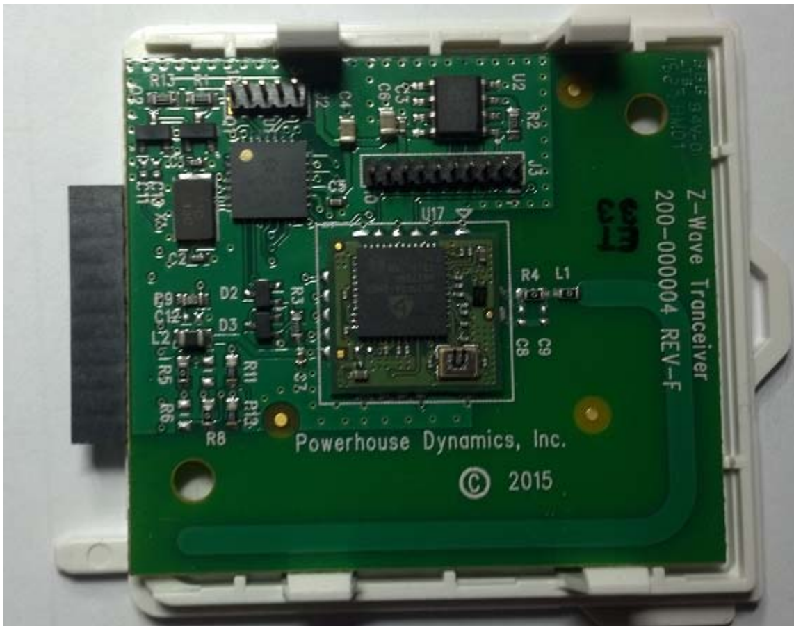
Z-Wave Module Assembly – ZM5202 chip assembly situated in the middle of the PCB, antenna running from top of PCB down right hand side. Host connection at the bottom.
