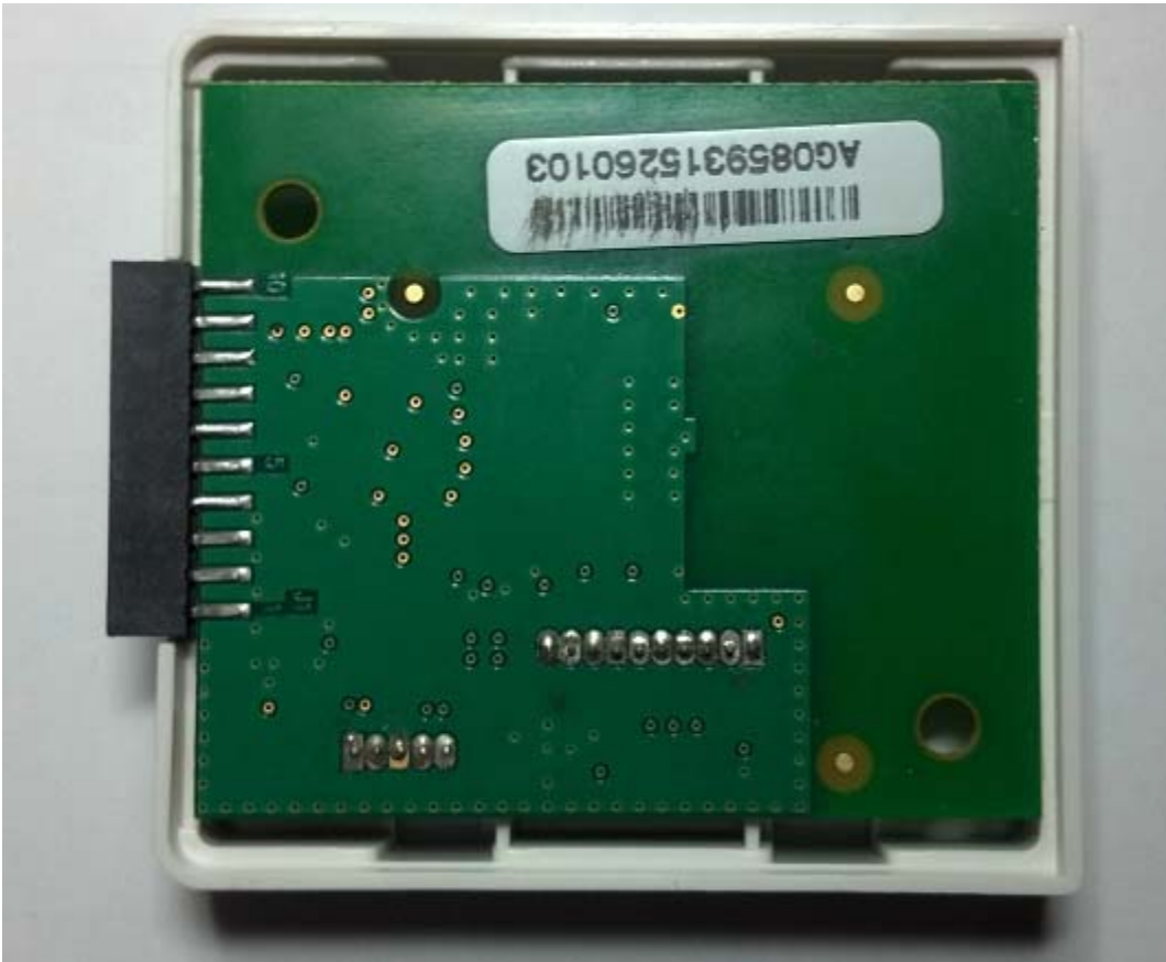
Rear of PCB showing Ground Plane
