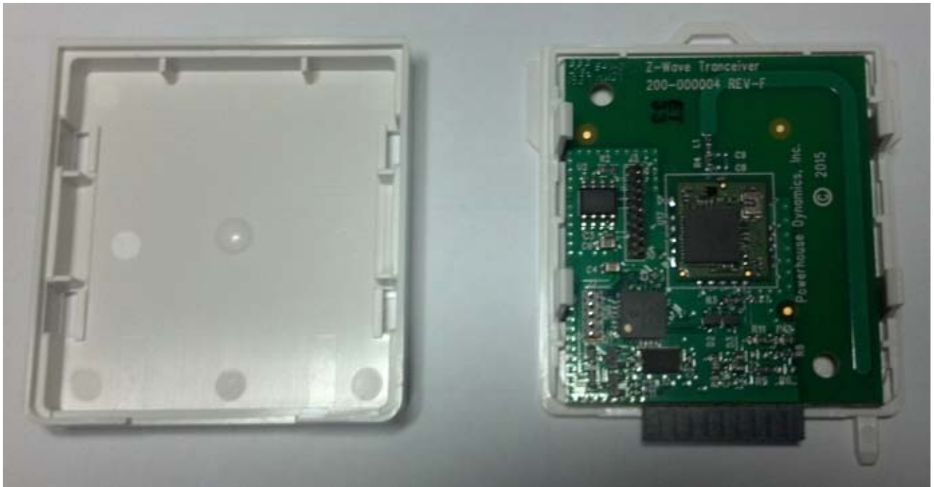
Z-Wave Module Assembly – ZM5202 chip assembly situated in the middle of the PCB, antenna running from top of PCB down right hand side. Host connection at the bottom.
