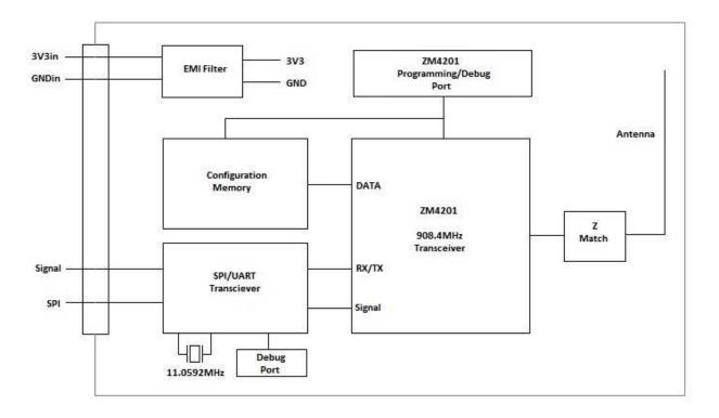
The Z-Wave Module is centered around the ZM4102 Z-Wave Transceiver programmed as a Z-Wave Controller, generating a carrier frequency of 908.4MH.
