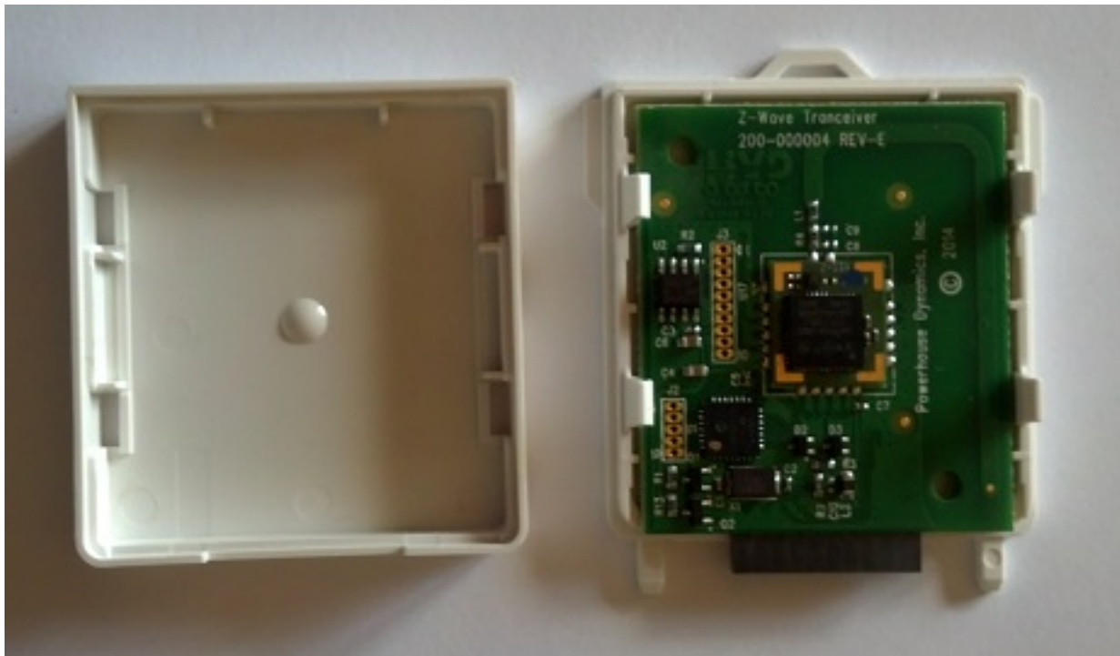
Z-Wave Module Assembly – ZM4102 chip assembly situated in the middle of the PCB, antenna running from top of PCB down right hand side. Host connection at the bottom.
