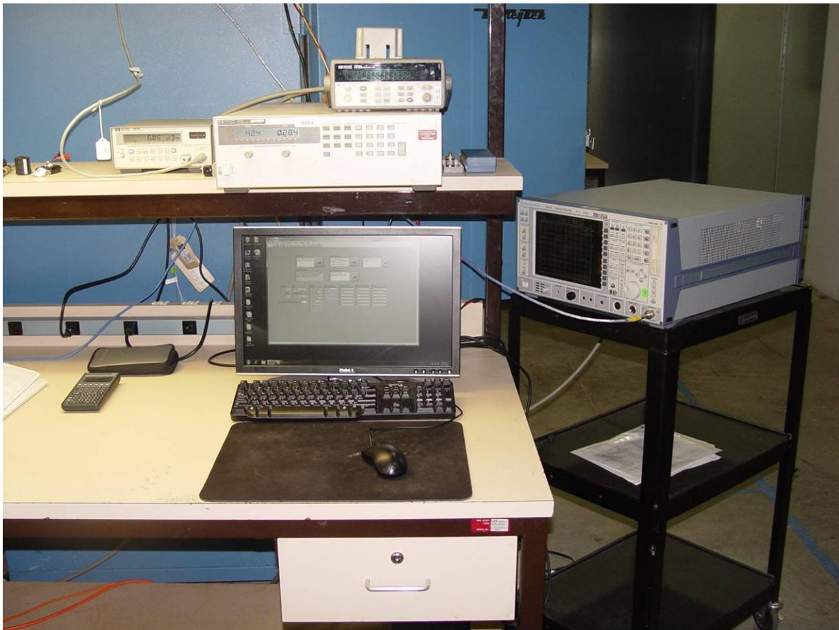
Transmitter Radiated Spurious Emission above 1 GHz
