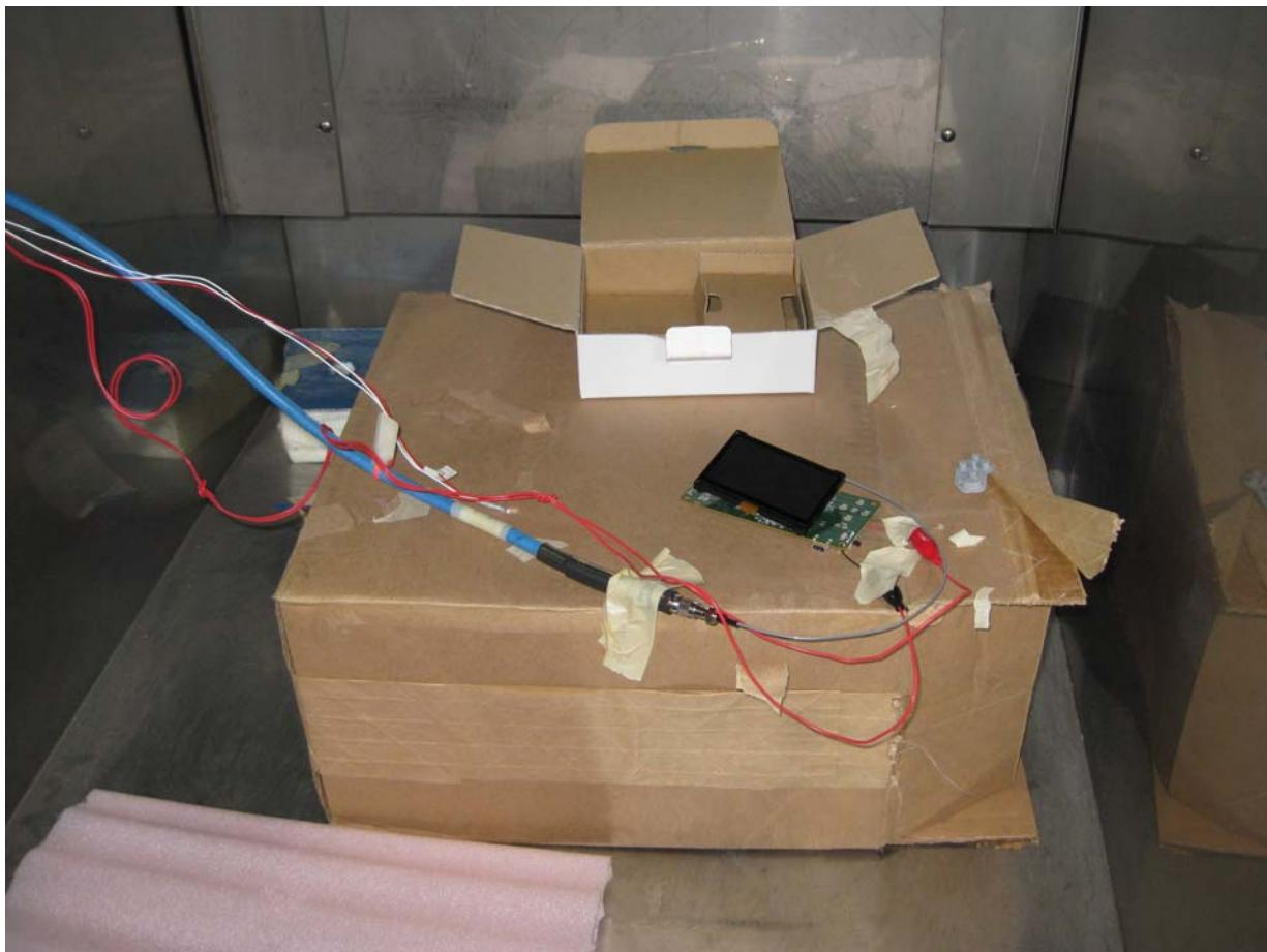
Conducted RF Emissions - Test Equipment
