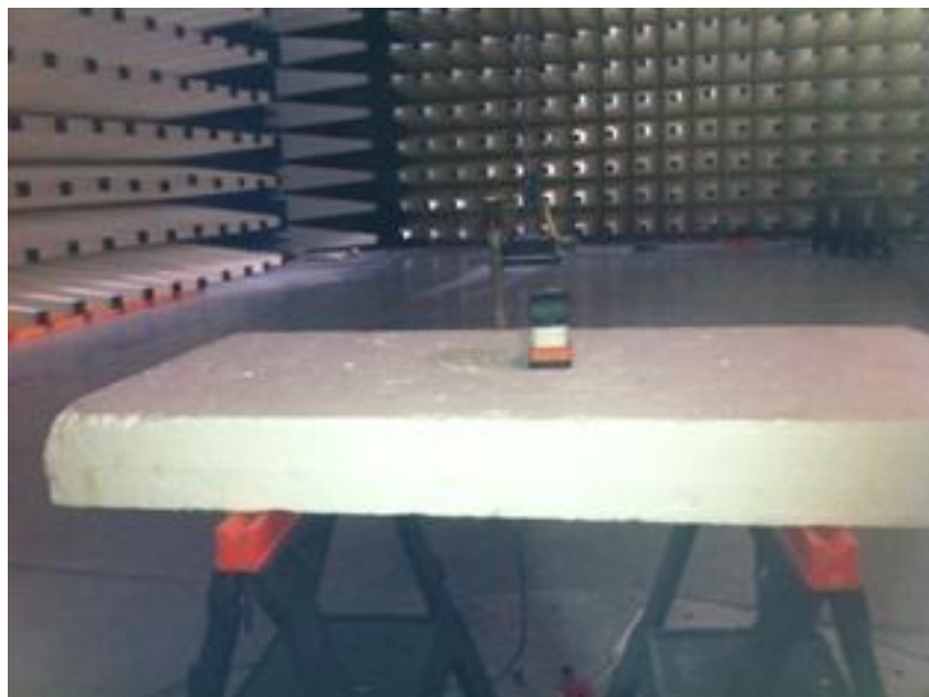
Figure 2: Radiated emissions setup above 1 GHz
