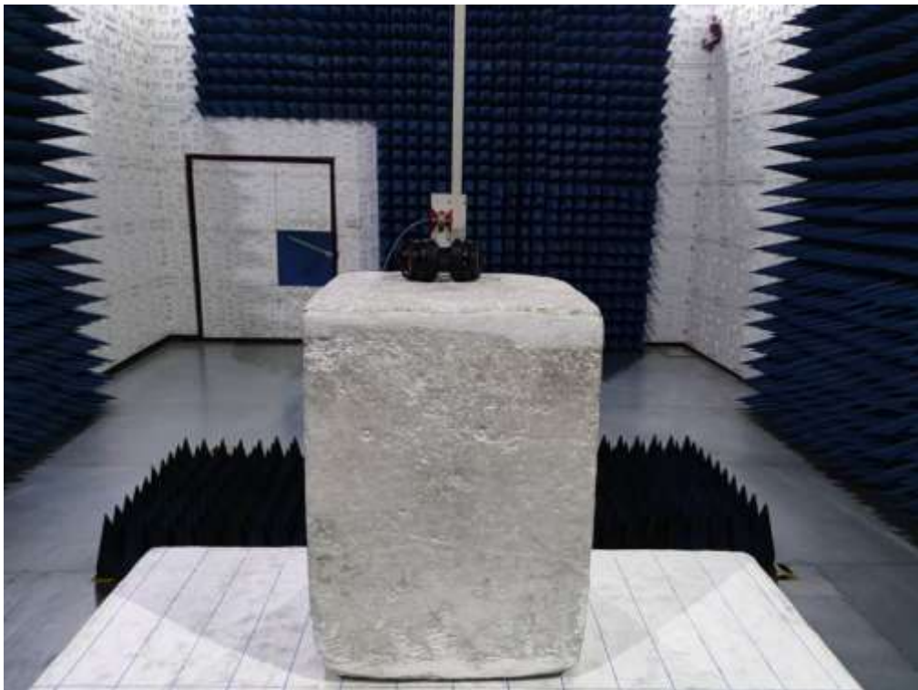
RADIATED EMISSION TEST SETUP ABOVE 1GHZ
