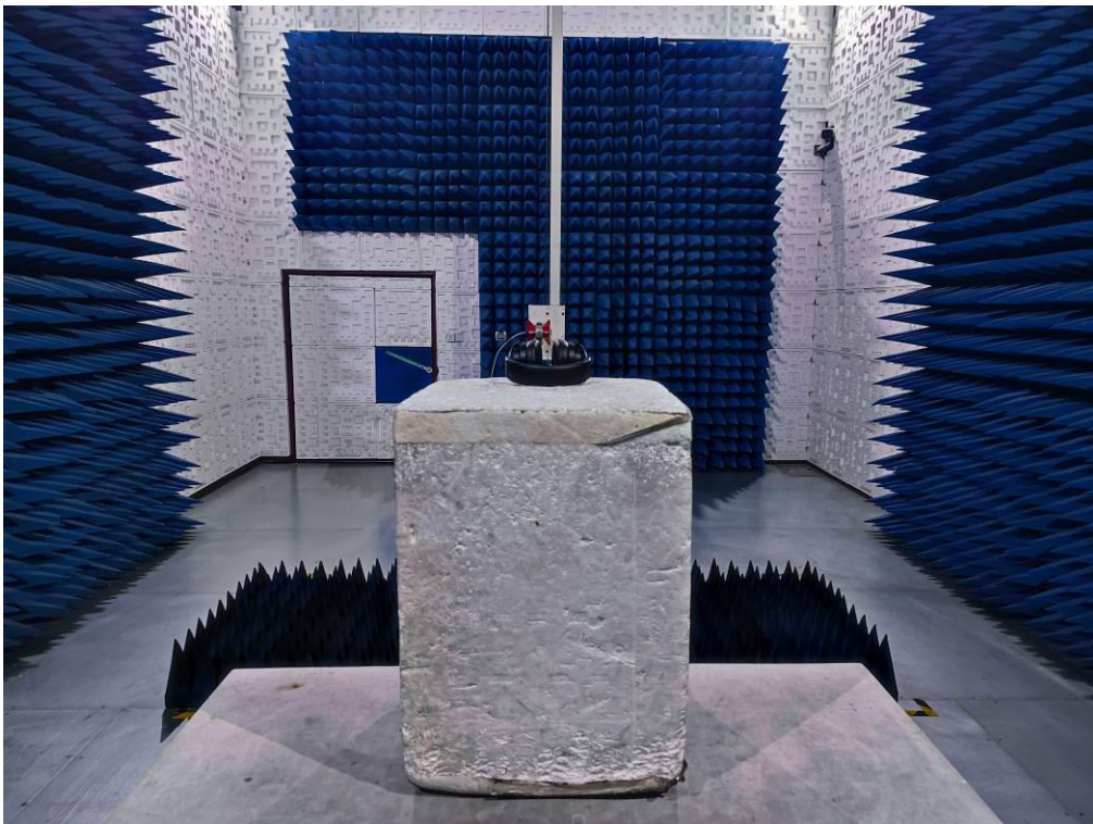
RADIATED EMISSION TEST SETUP ABOVE 1GHz
