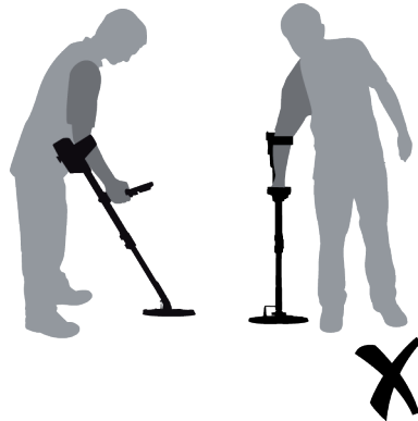
Shaft is too short
