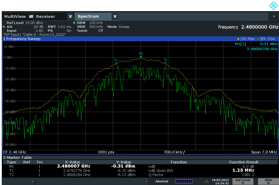
Graph 6-3: 6 dB bandwidth, 2480 MHz
