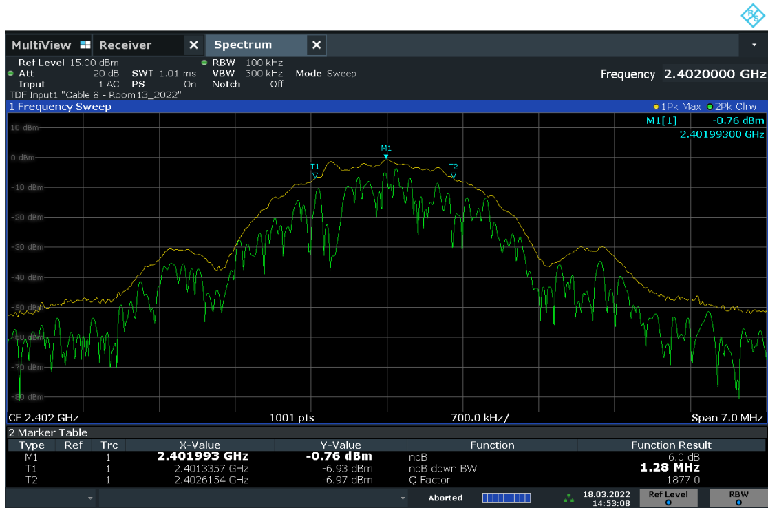
Graph 6-1: 6 dB bandwidth, 2402 MHz
