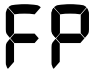
'FP' will appear on the Target ID display when Factory Presets are restored.
