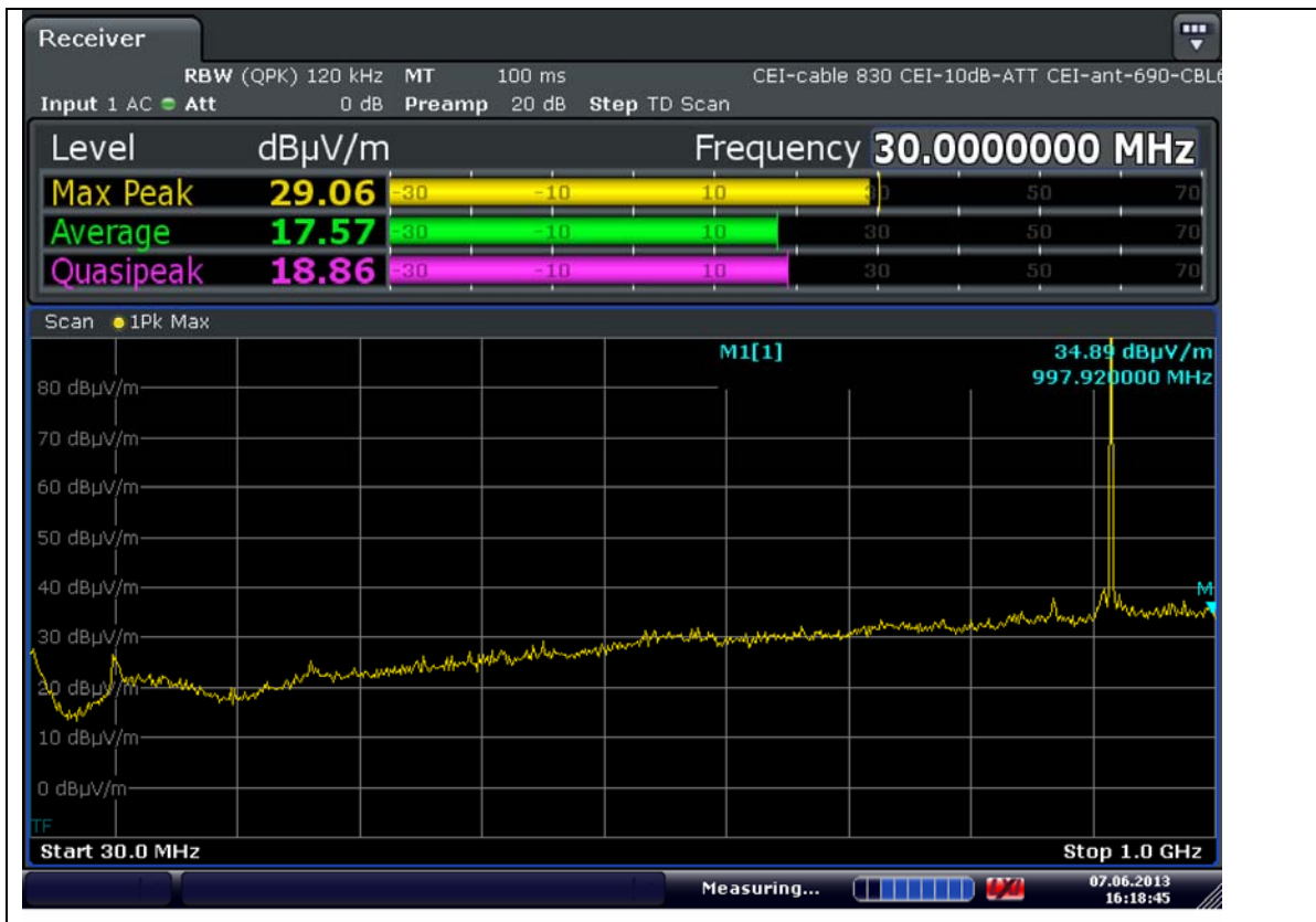
Fig 4 Scan 30 MHz- 1GHz Horizontal 3 metres Anechoic Chamber
