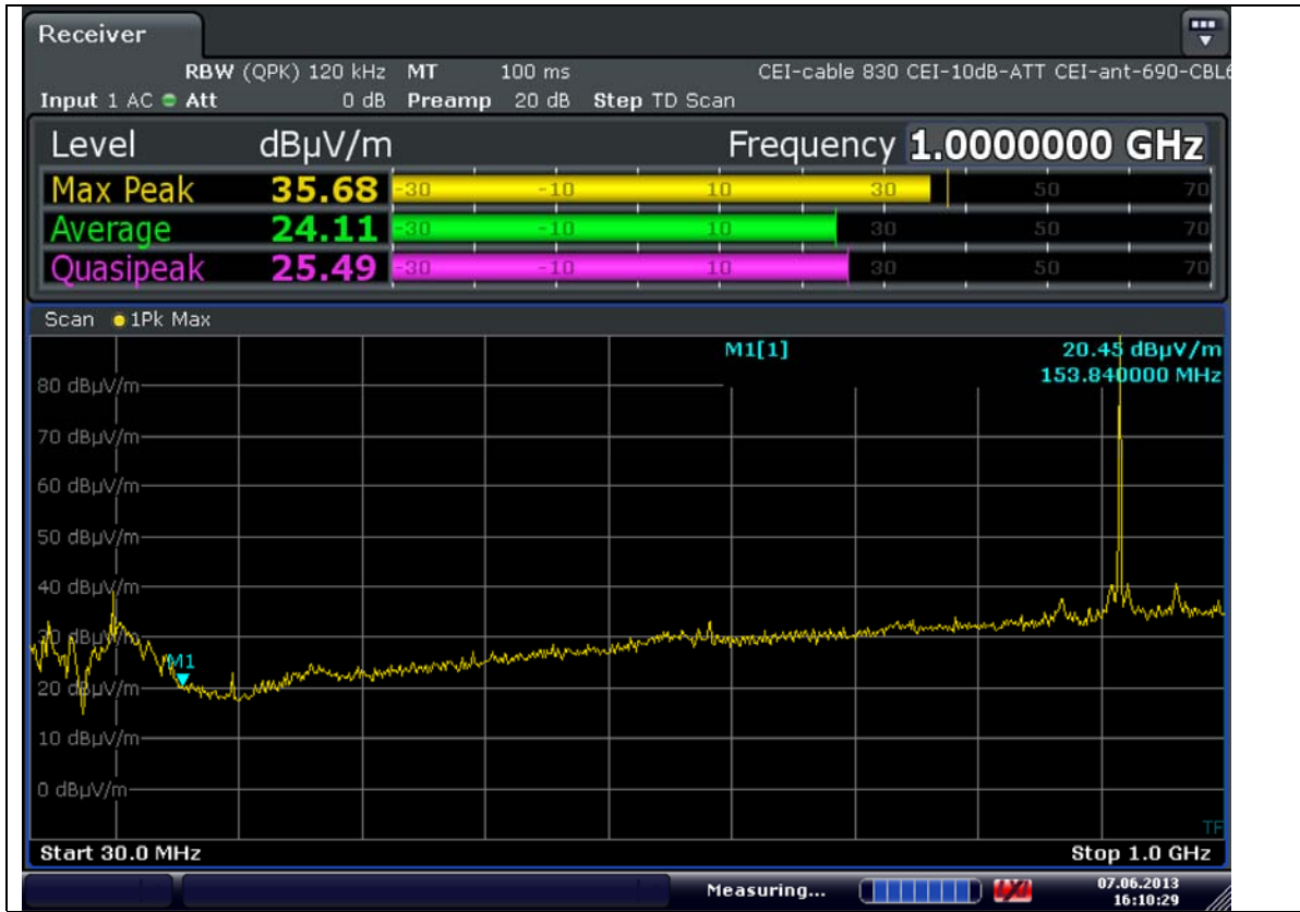
Fig 3 Scan 30 MHz - 1GHz Vertical 3 metres Anechoic Chamber
