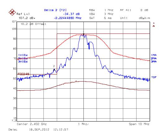
**Plot 5.7.4.2.** Band-Edge RF Radiated Emissions @ 3 m, Continuous Mode Low End of Frequency Band, 2402 MHz, Rx Antenna Orientation: Horizontal
