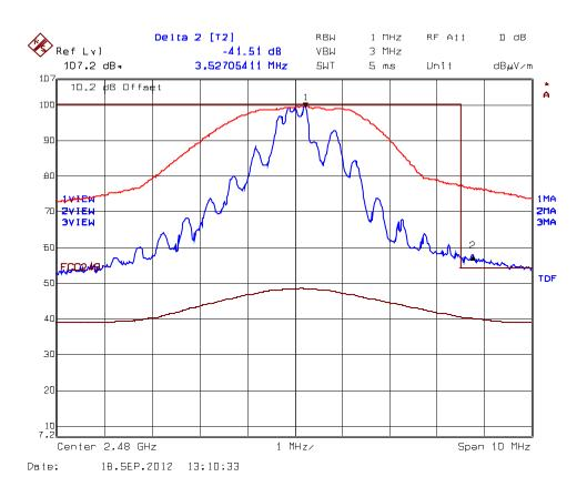
**Plot 5.7.4.8.** Band-Edge RF Radiated Emissions @ 3 m, Continuous Mode High End of Frequency Band, 2480 MHz, Rx Antenna Orientation: Vertical
