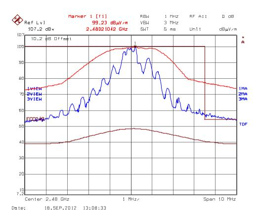
**Plot 5.7.4.7.** Band-Edge RF Radiated Emissions @ 3 m, Continuous Mode High End of Frequency Band, 2480 MHz, Rx Antenna Orientation: Vertical
