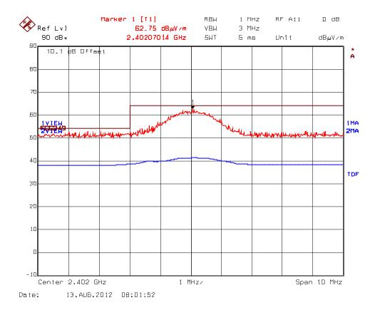
**Plot 5.9.4.2.** Band-Edge RF Radiated Emissions @ 3 m, Continuous Mode Low End of Frequency Band, 2402 MHz, Rx Antenna Orientation: Vertical
