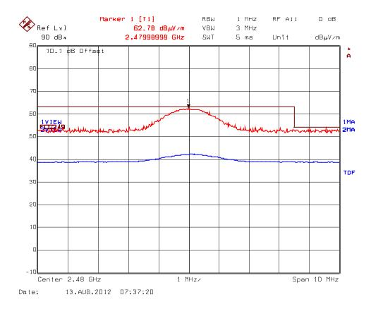
**Plot 5.9.4.4.** Band-Edge RF Radiated Emissions @ 3 m, Continuous Mode High End of Frequency Band, 2480 MHz, Rx Antenna Orientation: Vertical
