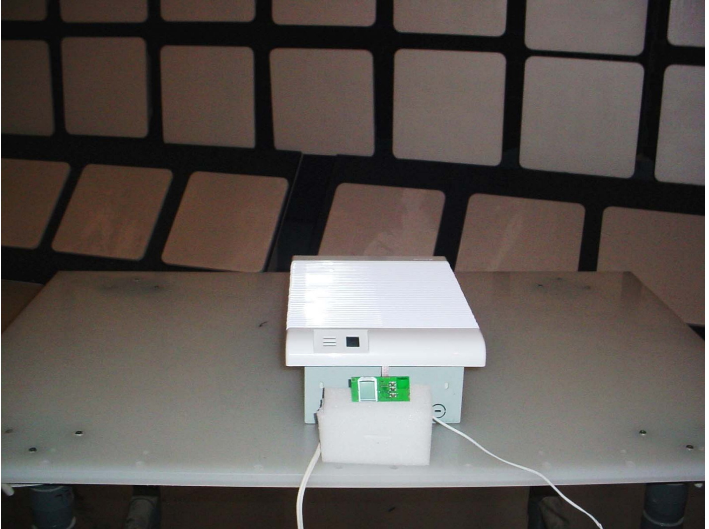
Tx Radiated Emissions at 3 m, Orthogonal Position 2
