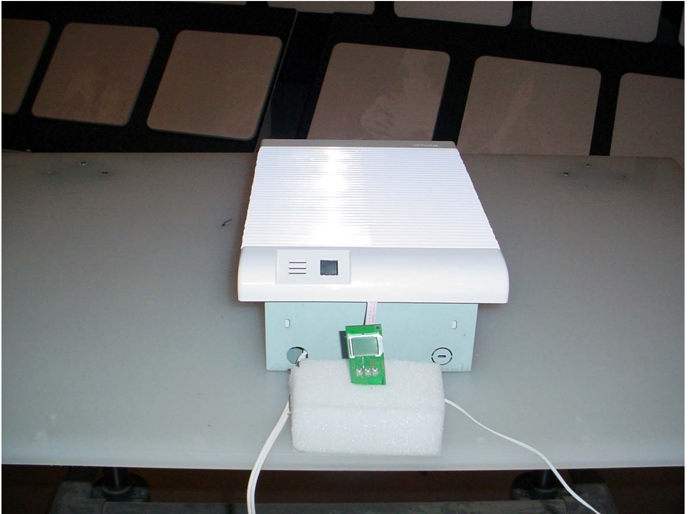
Tx Radiated Emissions at 3 m, Orthogonal Position 3
