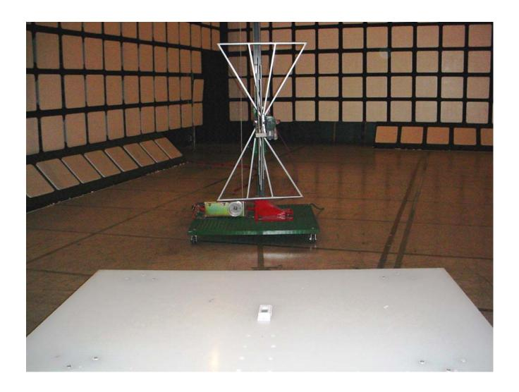
Tx Radiated Emissions at 3 m, Orthogonal Position 2
