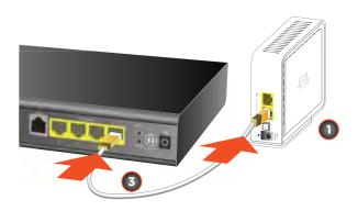
Plug one of the power adapters 2 first into the product and then to a power socket. Turn on the unit.
