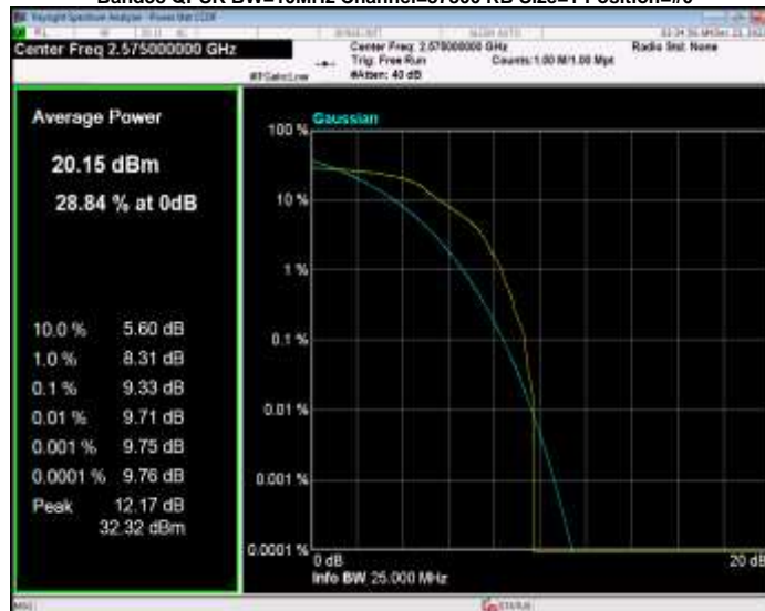
Band38 QPSK BW=10MHz Channel=37800 RB Size=1 Position=#0
