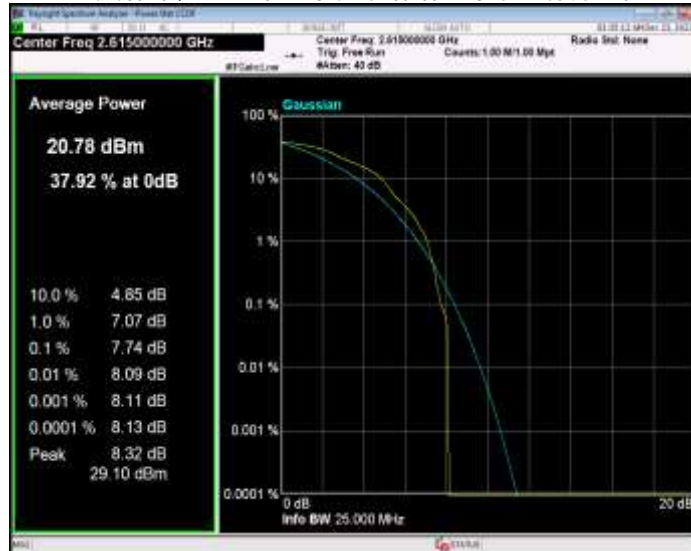
Band38 16QAM BW=15MHz Channel=37825 RB Size=1 Position=#0
