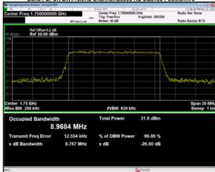
Band4 QPSK BW=10MHz Channel=20350 RB Size=50 Position=#0
