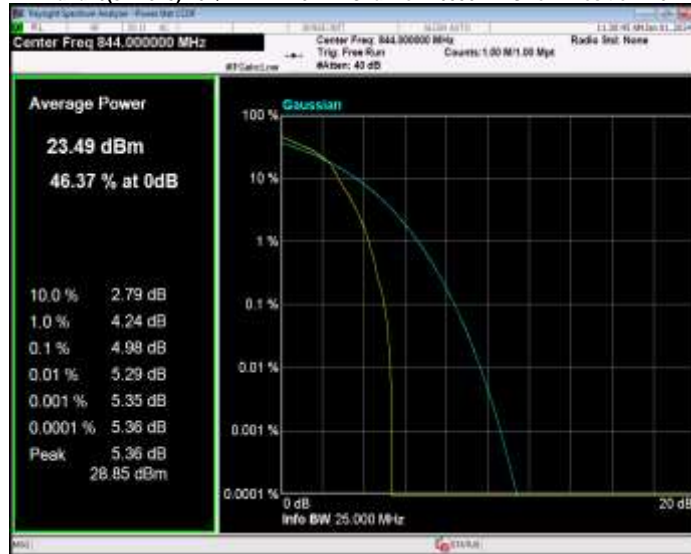
Band26(824-849) 16QAM BW=15MHz Channel=26865 RB Size=1 Position=#0
