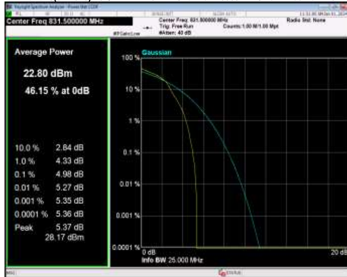
Band26(824-849) 16QAM BW=15MHz Channel=26915 RB Size=1 Position=#0
