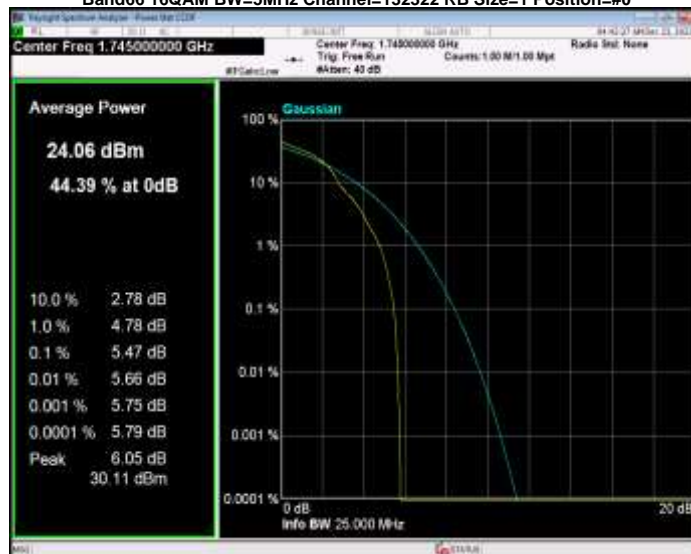
Band66 16QAM BW=5MHz Channel=132322 RB Size=1 Position=#0
