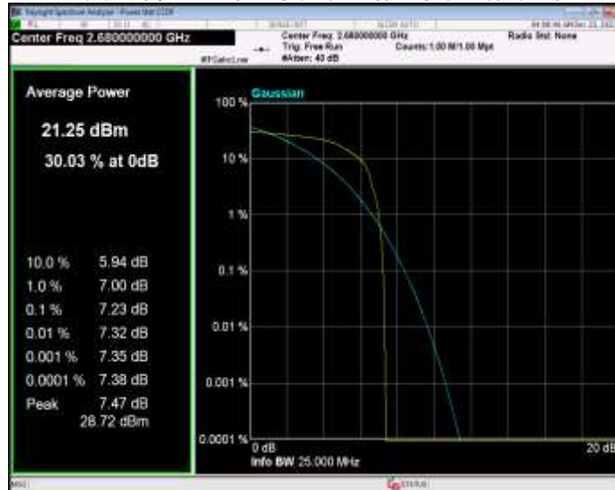
Band41 16QAM BW=5MHz Channel=39675 RB Size=1 Position=#0
