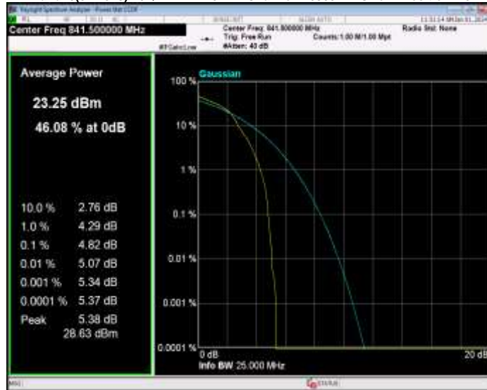
Band26(824-849) 16QAM BW=3MHz Channel=26805 RB Size=1 Position=#0
