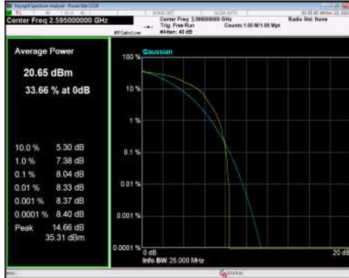
Band38 16QAM BW=10MHz Channel=38200 RB Size=1 Position=#0
