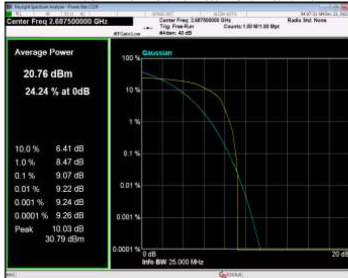
Band41 QPSK BW=10MHz Channel=39700 RB Size=1 Position=#0
