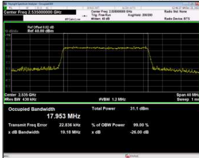
Band7 16QAM BW=20MHz Channel=21350 RB Size=100 Position=#0
