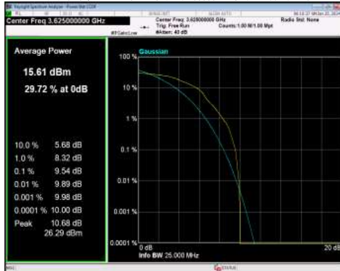
Band48 16QAM BW=5MHz Channel=55990 RB Size=1 Position=#0
