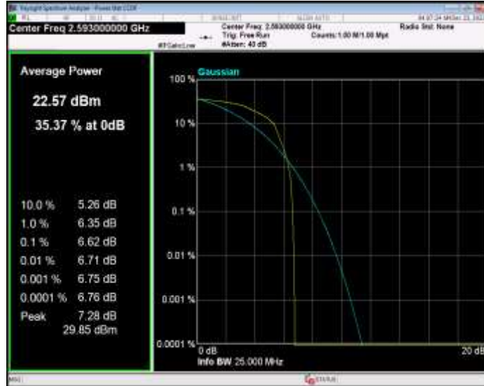
Band41 16QAM BW=5MHz Channel=41565 RB Size=1 Position=#0
