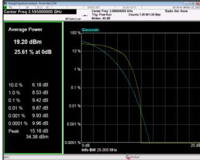
Band38 16QAM BW=5MHz Channel=38225 RB Size=1 Position=#0
