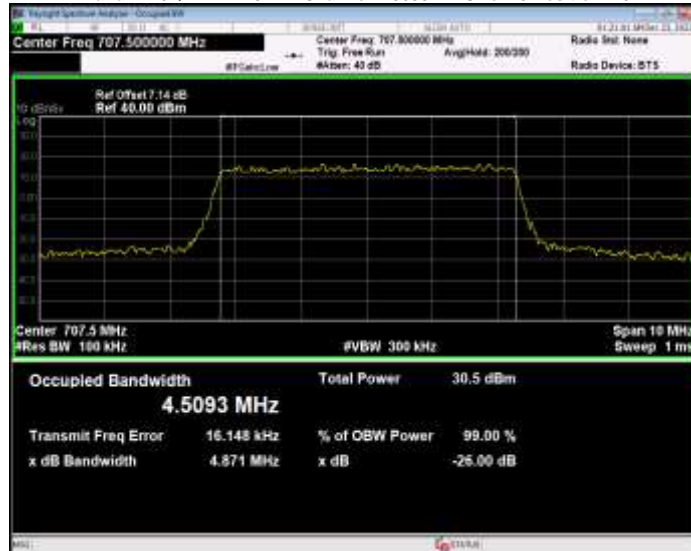
Band12 16QAM BW=5MHz Channel=23155 RB Size=25 Position=#0
