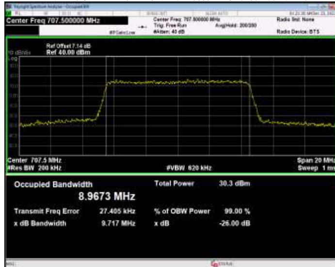
Band12 16QAM BW=10MHz Channel=23130 RB Size=50 Position=#0
