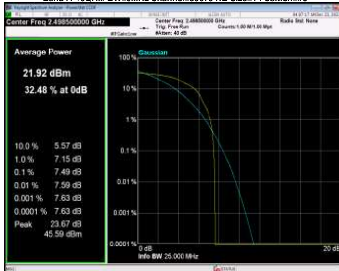
Band41 16QAM BW=5MHz Channel=39675 RB Size=1 Position=#0
