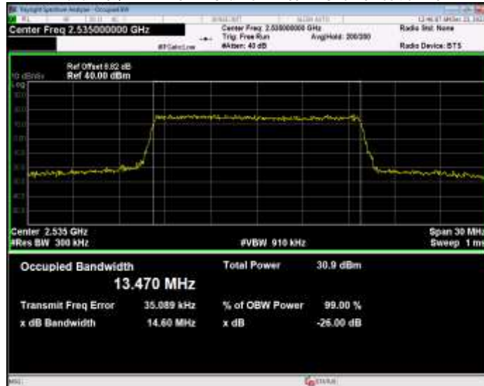
Band7 16QAM BW=15MHz Channel=21375 RB Size=75 Position=#0
