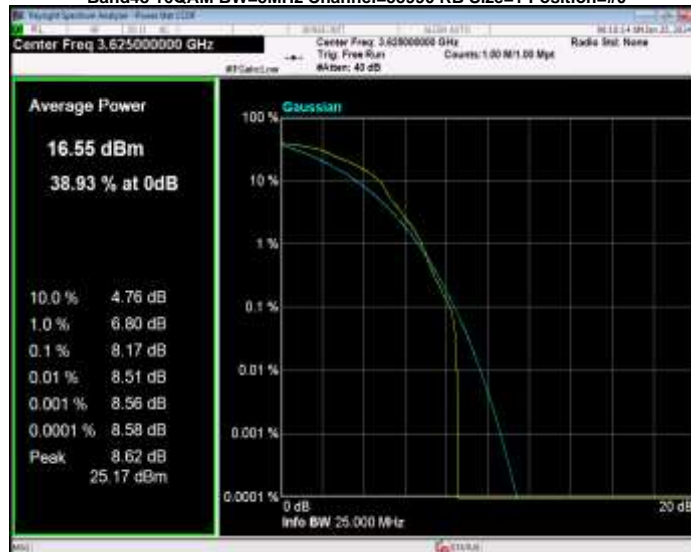
Band48 16QAM BW=5MHz Channel=55990 RB Size=1 Position=#0
