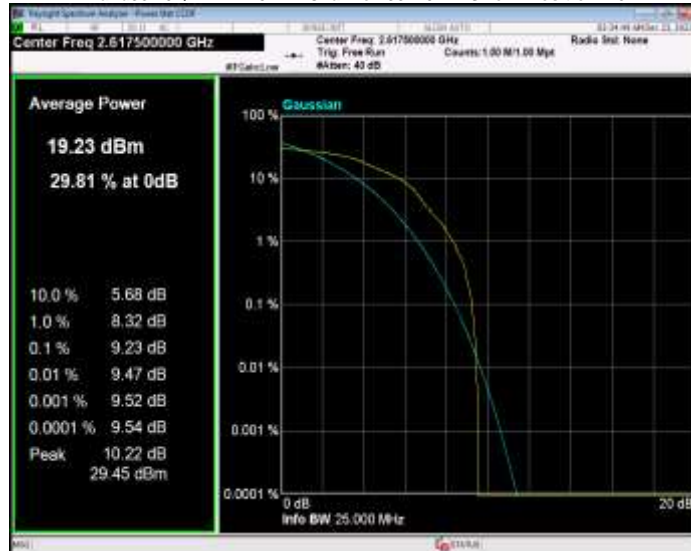
Band38 QPSK BW=10MHz Channel=37800 RB Size=1 Position=#0
