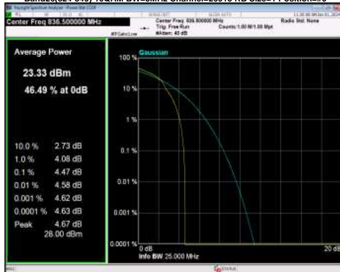
Band26(824-849) 16QAM BW=5MHz Channel=26915 RB Size=1 Position=#0
