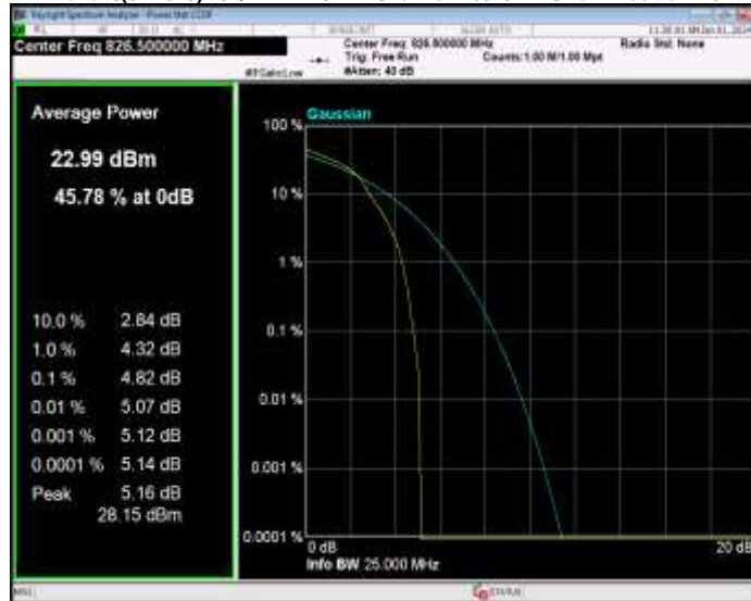
Band26(824-849) 16QAM BW=5MHz Channel=26915 RB Size=1 Position=#0
