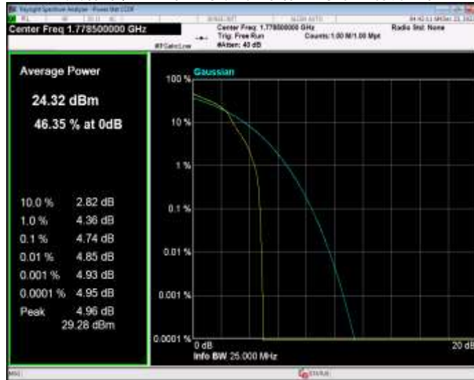
Band66 16QAM BW=5MHz Channel=131997 RB Size=1 Position=#0
