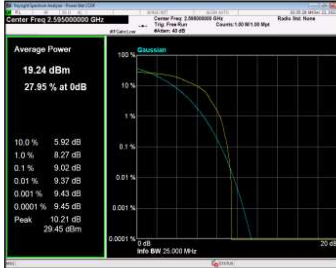
Band38 16QAM BW=15MHz Channel=38175 RB Size=1 Position=#0
