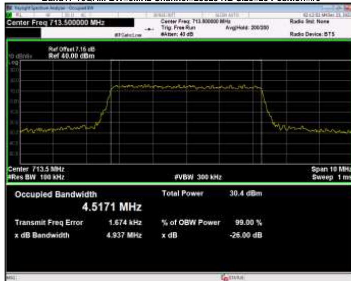
Band17 QPSK BW=10MHz Channel=23780 RB Size=50 Position=#0
