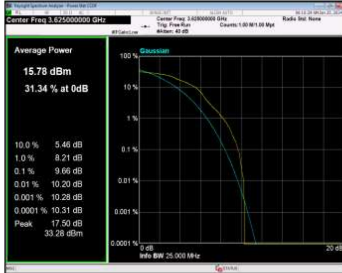
Band48 16QAM BW=20MHz Channel=55990 RB Size=1 Position=#0
