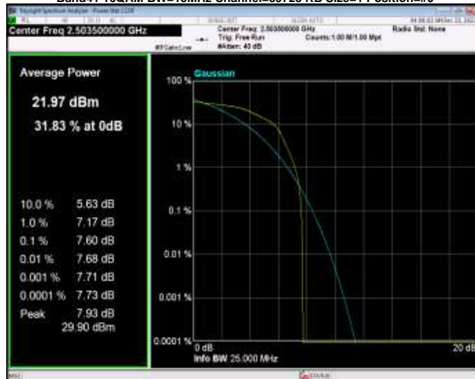
Band41 16QAM BW=15MHz Channel=39725 RB Size=1 Position=#0
