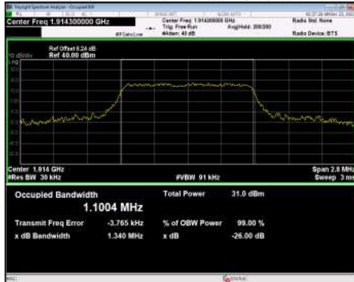
Band25 16QAM BW=10MHz Channel=26090 RB Size=50 Position=#0
