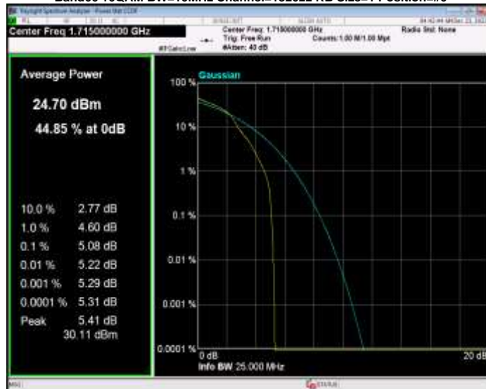
Band66 16QAM BW=10MHz Channel=132322 RB Size=1 Position=#0
