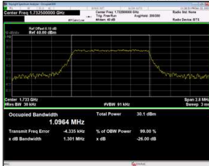
Band4 16QAM BW=1.4MHz Channel=20393 RB Size=6 Position=#0
