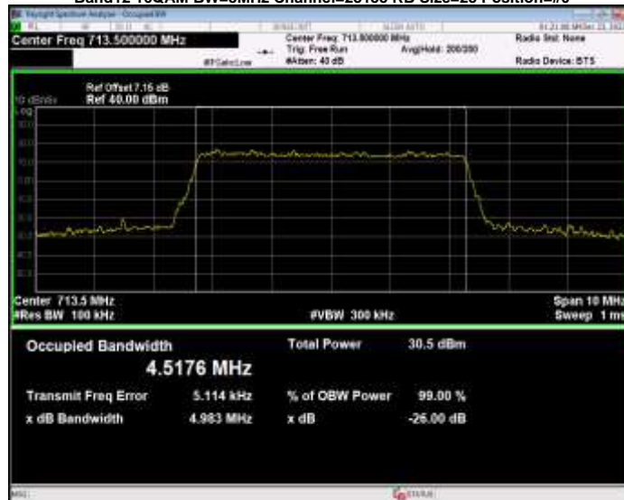
Band12 16QAM BW=5MHz Channel=23155 RB Size=25 Position=#0
