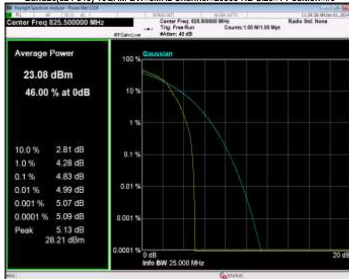
Band26(824-849) 16QAM BW=3MHz Channel=26915 RB Size=1 Position=#0
