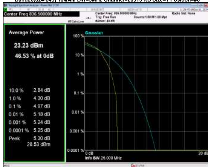
Band26(824-849) 16QAM BW=3MHz Channel=26915 RB Size=1 Position=#0
