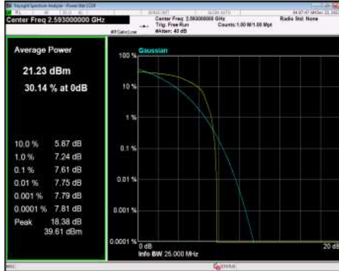
Band41 16QAM BW=10MHz Channel=41540 RB Size=1 Position=#0
