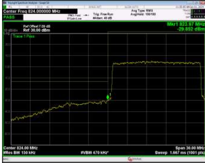
Band26(824-849) QPSK BW=15MHz Channel=26965 RB Size=75 Position=#0
