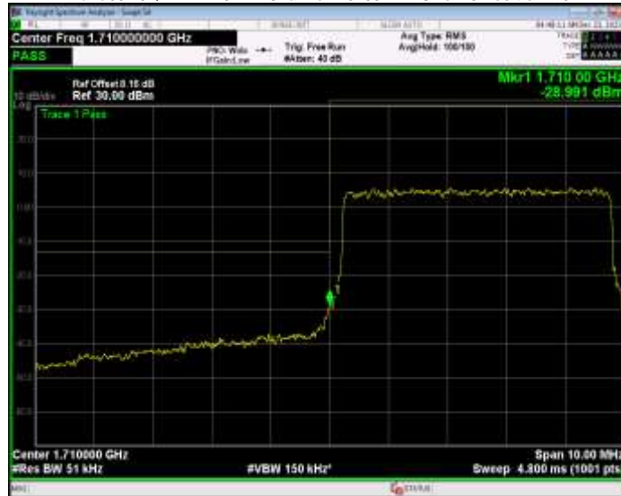
Band66 16QAM BW=5MHz Channel=132647 RB Size=25 Position=#0
