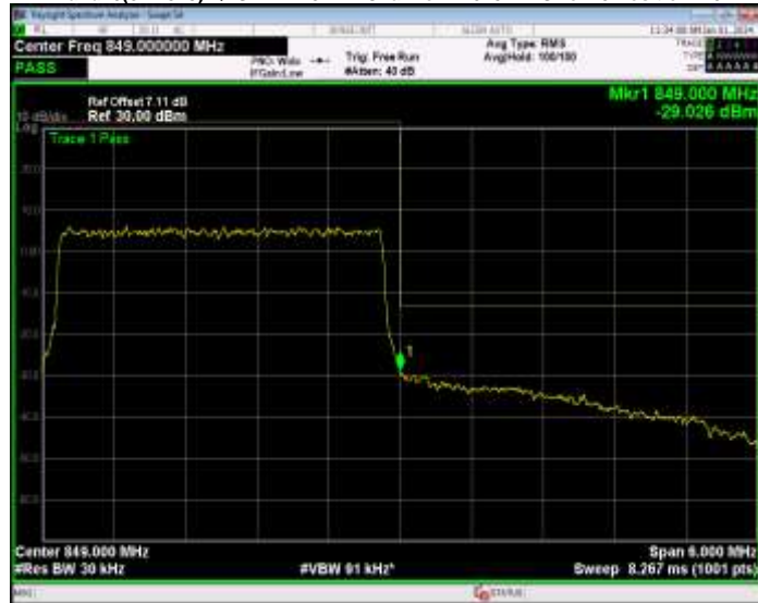
Band26(824-849) QPSK BW=5MHz Channel=26815 RB Size=25 Position=#0
