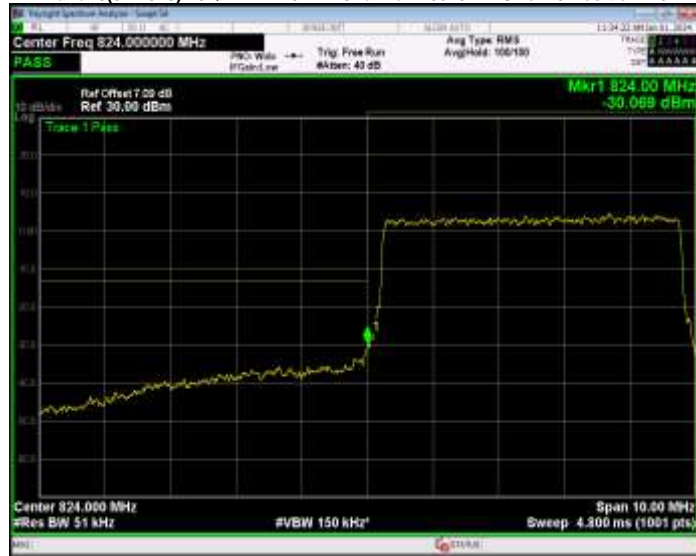
Band26(824-849) 16QAM BW=5MHz Channel=27015 RB Size=25 Position=#0
