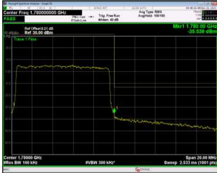
Band66 16QAM BW=15MHz Channel=132047 RB Size=75 Position=#0
