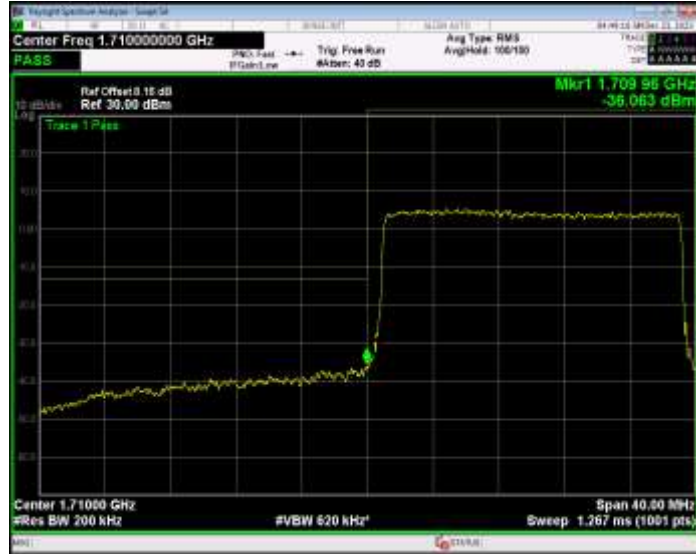
Band66 16QAM BW=20MHz Channel=132572 RB Size=100 Position=#0
