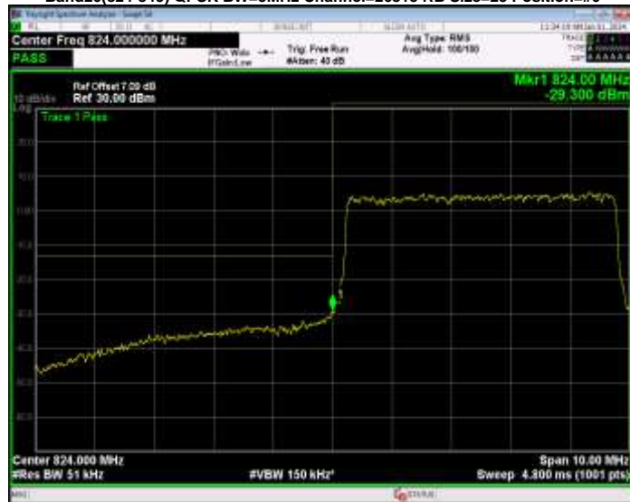
Band26(824-849) QPSK BW=5MHz Channel=27015 RB Size=25 Position=#0
