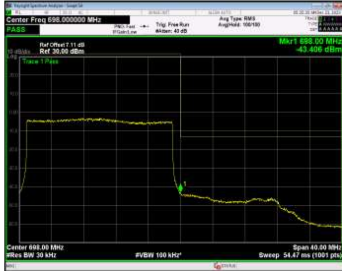
Band71 QPSK BW=5MHz Channel=133147 RB Size=25 Position=#0
