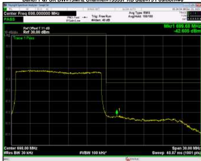
Band71 QPSK BW=15MHz Channel=133397 RB Size=75 Position=#0
