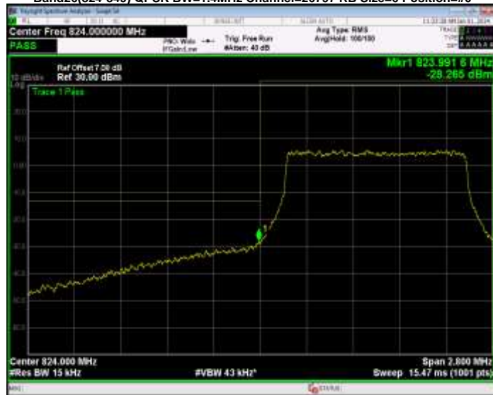
Band26(824-849) QPSK BW=1.4MHz Channel=26797 RB Size=6 Position=#0
