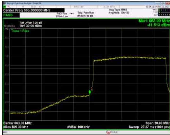
Band71 16QAM BW=10MHz Channel=133422 RB Size=50 Position=#0
