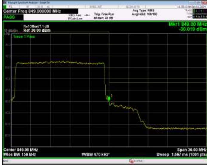
Band26(824-849) QPSK BW=3MHz Channel=26805 RB Size=15 Position=#0
