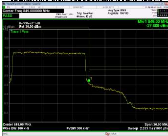
Band26(824-849) QPSK BW=10MHz Channel=26990 RB Size=50 Position=#0
