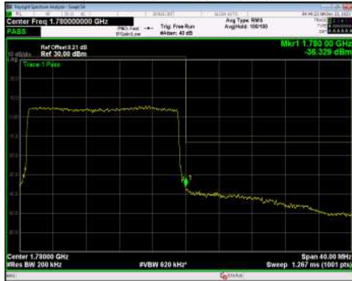
Band66 16QAM BW=3MHz Channel=131987 RB Size=15 Position=#0
