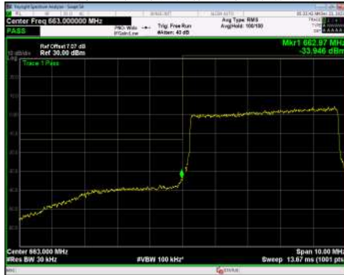
Band71 16QAM BW=5MHz Channel=133447 RB Size=25 Position=#0
