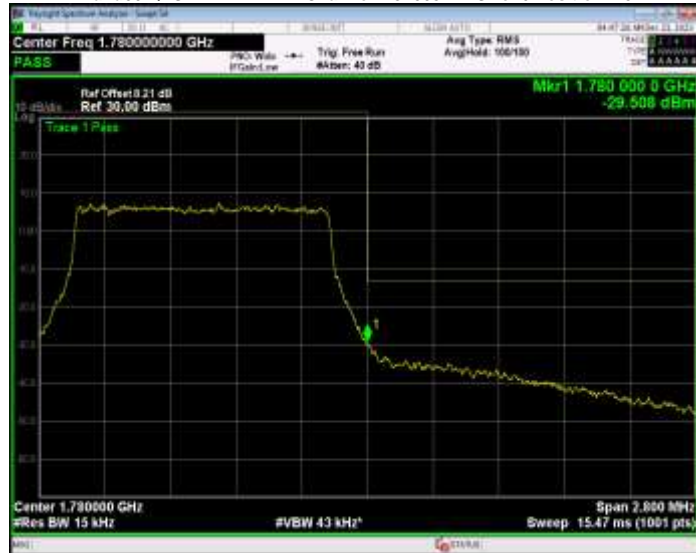
Band66 QPSK BW=10MHz Channel=132022 RB Size=50 Position=#0
