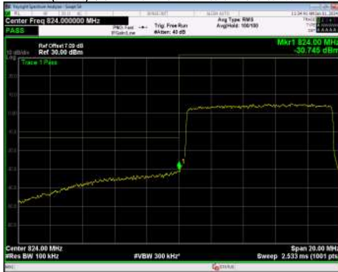
Band26(824-849) QPSK BW=10MHz Channel=26990 RB Size=50 Position=#0
