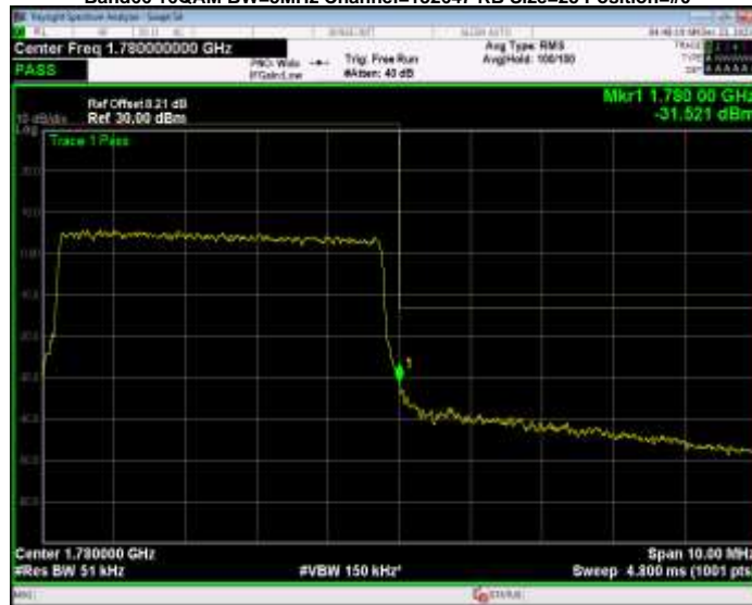
Band66 16QAM BW=5MHz Channel=132647 RB Size=25 Position=#0
