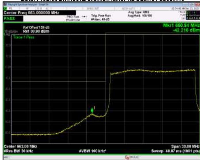
Band71 16QAM BW=15MHz Channel=133197 RB Size=75 Position=#0
