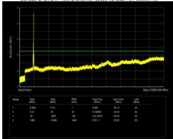
Band38 QPSK BW=15MHz Channel=38175 RB Size=75 Position=#0
