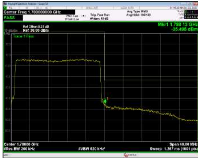
Band66 QPSK BW=3MHz Channel=131987 RB Size=15 Position=#0
