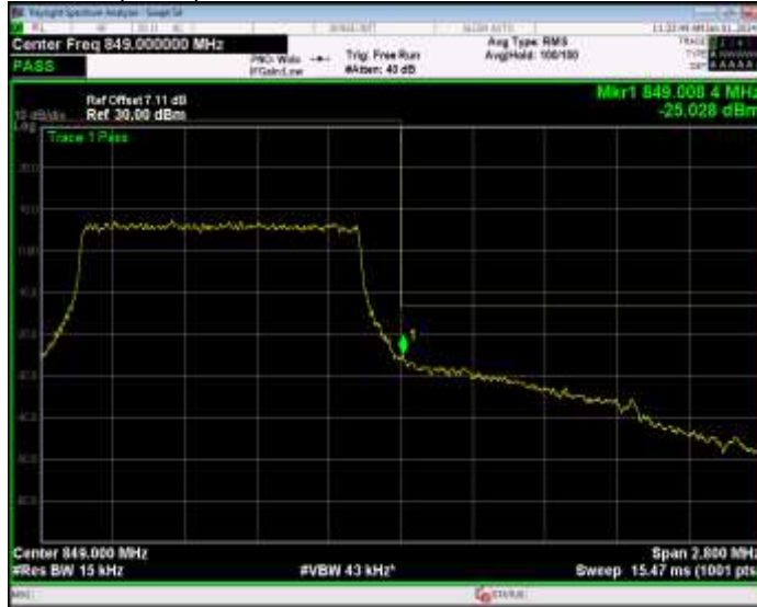
Band26(824-849) QPSK BW=10MHz Channel=26840 RB Size=50 Position=#0
