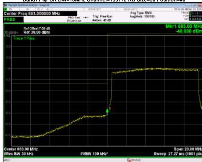
Band71 QPSK BW=10MHz Channel=133172 RB Size=50 Position=#0
