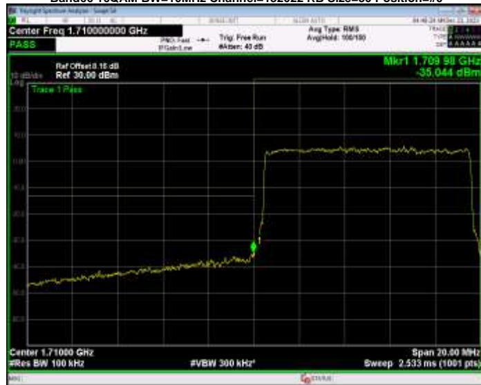
Band66 16QAM BW=10MHz Channel=132022 RB Size=50 Position=#0
