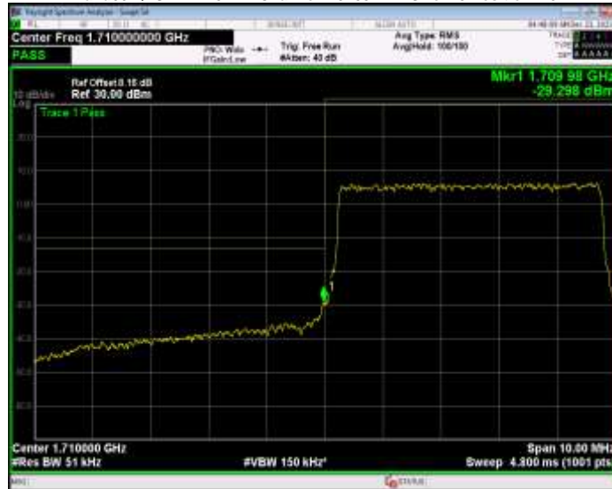
Band66 QPSK BW=5MHz Channel=132647 RB Size=25 Position=#0
