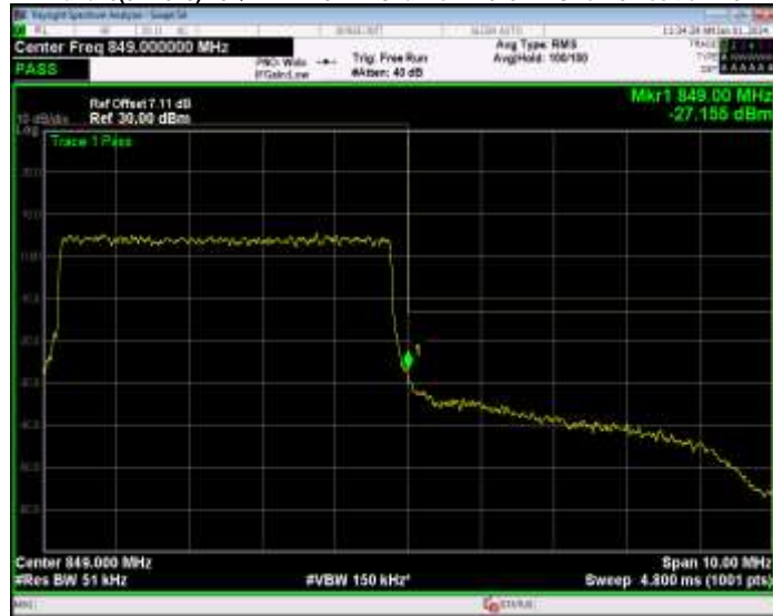
Band26(824-849) QPSK BW=1.4MHz Channel=26797 RB Size=6 Position=#0
