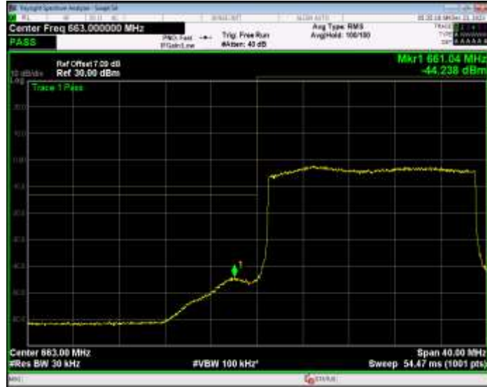
Band71 QPSK BW=20MHz Channel=133372 RB Size=100 Position=#0
