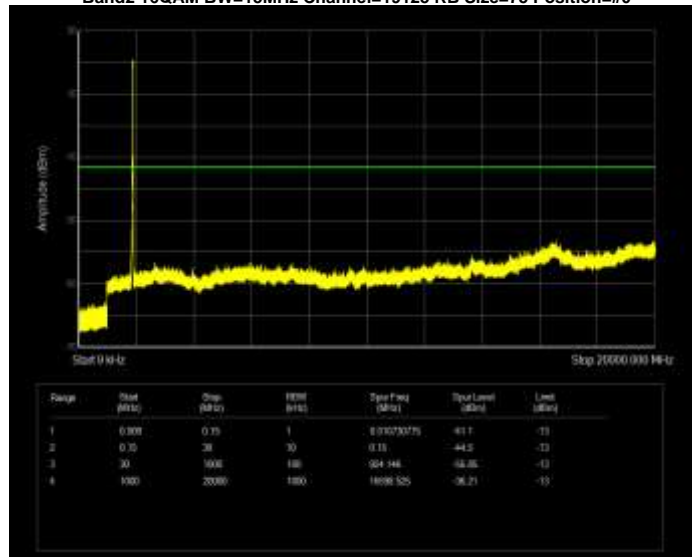
Band2 16QAM BW=15MHz Channel=19125 RB Size=75 Position=#0
