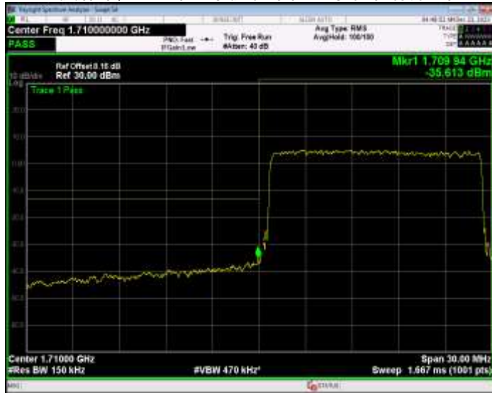
Band66 16QAM BW=15MHz Channel=132597 RB Size=75 Position=#0
