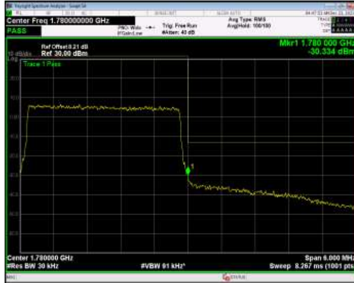
Band66 QPSK BW=5MHz Channel=131997 RB Size=25 Position=#0
