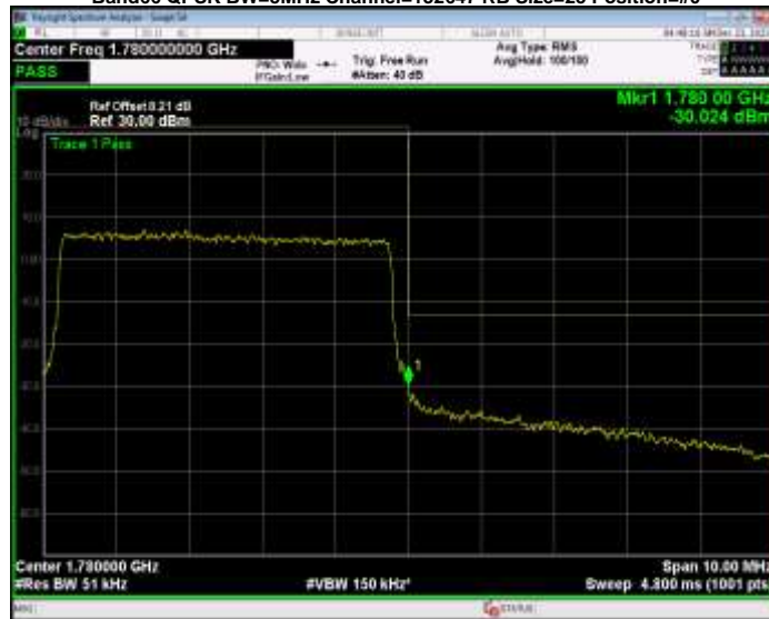
Band66 QPSK BW=5MHz Channel=132647 RB Size=25 Position=#0
