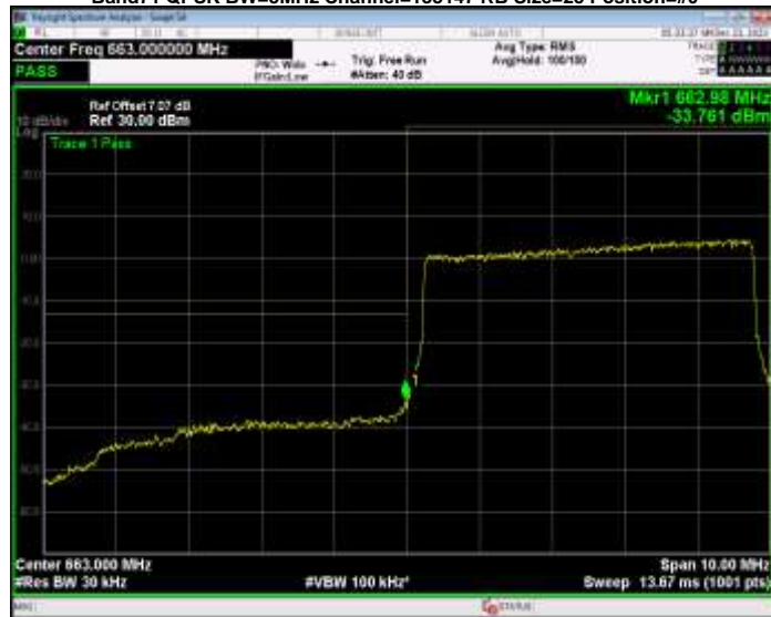
Band71 QPSK BW=5MHz Channel=133147 RB Size=25 Position=#0
