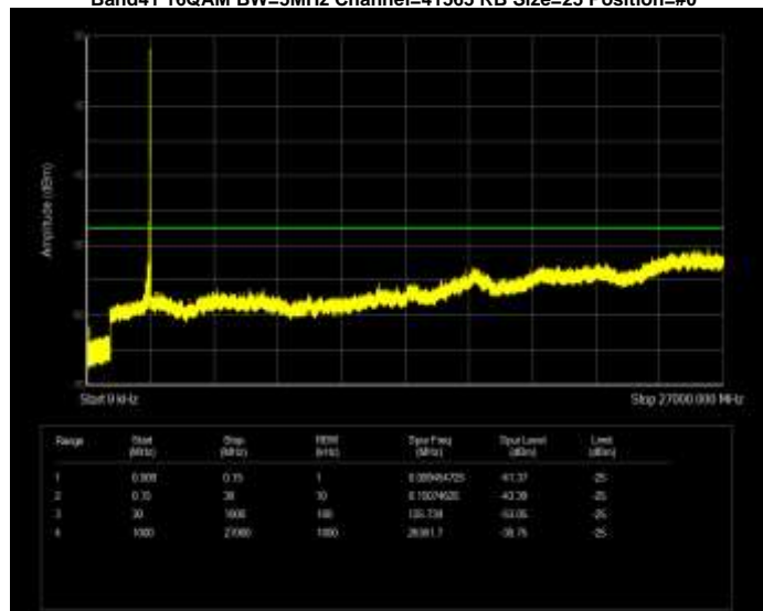
Band41 16QAM BW=5MHz Channel=41565 RB Size=25 Position=#0
