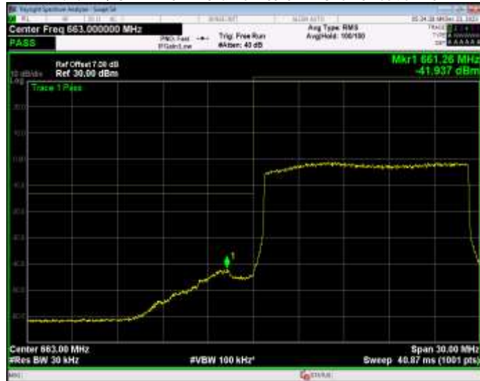
Band71 QPSK BW=15MHz Channel=133397 RB Size=75 Position=#0
