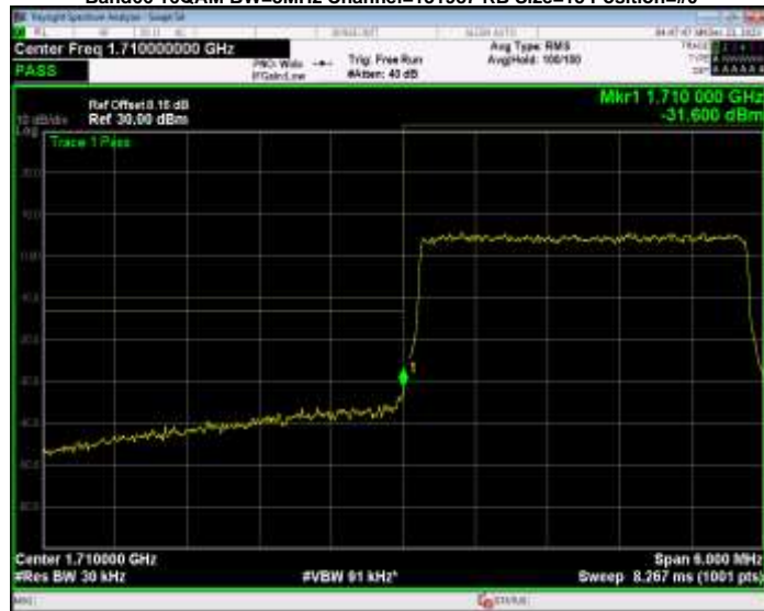
Band66 16QAM BW=3MHz Channel=131987 RB Size=15 Position=#0
