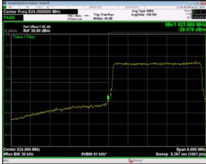
Band26(824-849) QPSK BW=3MHz Channel=26805 RB Size=15 Position=#0
