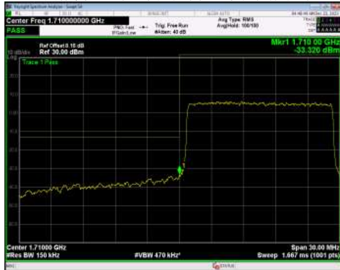
Band66 QPSK BW=15MHz Channel=132597 RB Size=75 Position=#0
