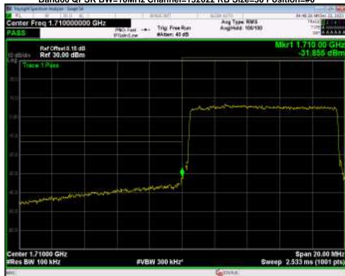
Band66 QPSK BW=10MHz Channel=132022 RB Size=50 Position=#0
