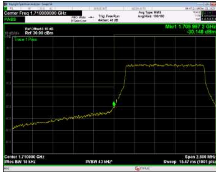
Band66 16QAM BW=1.4MHz Channel=132665 RB Size=6 Position=#0
