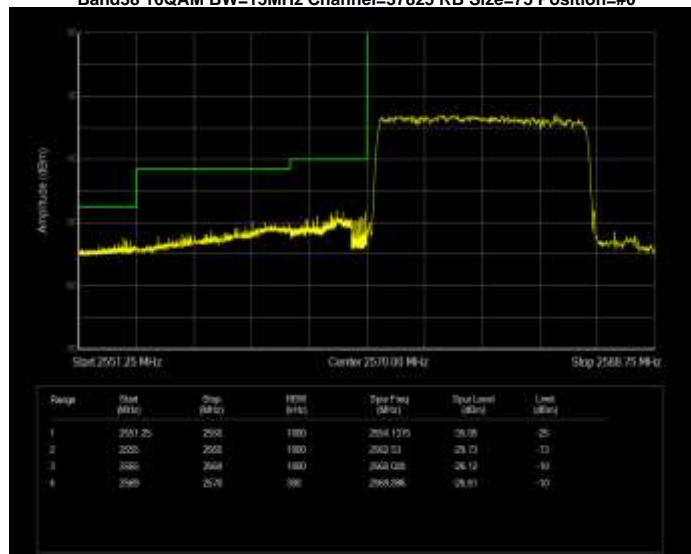
Band38 16QAM BW=15MHz Channel=37825 RB Size=75 Position=#0
