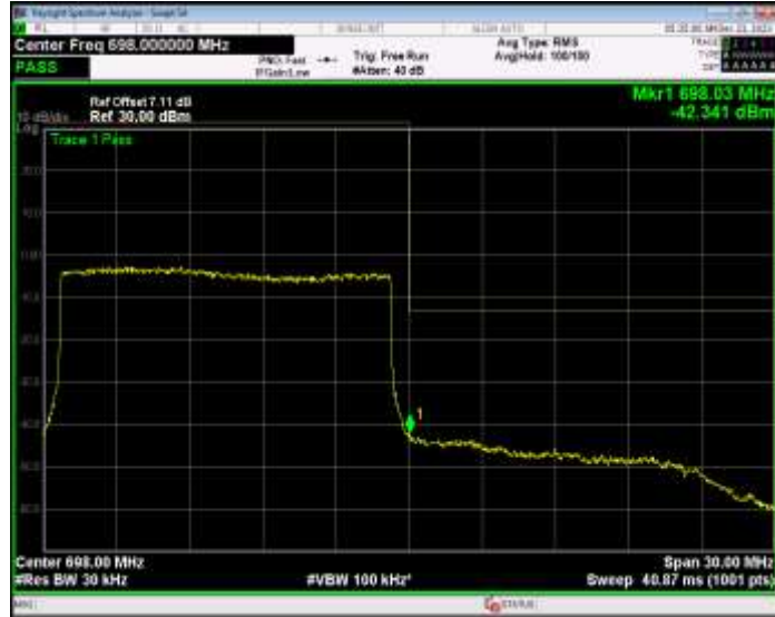
Band71 16QAM BW=20MHz Channel=133222 RB Size=100 Position=#0
