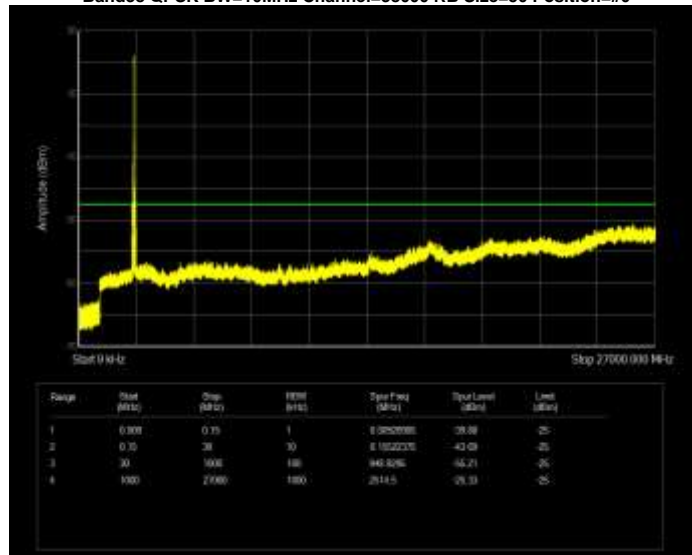
Band38 QPSK BW=10MHz Channel=38200 RB Size=50 Position=#0
