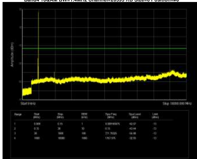
Band4 16QAM BW=1.4MHz Channel=20393 RB Size=6 Position=#0
