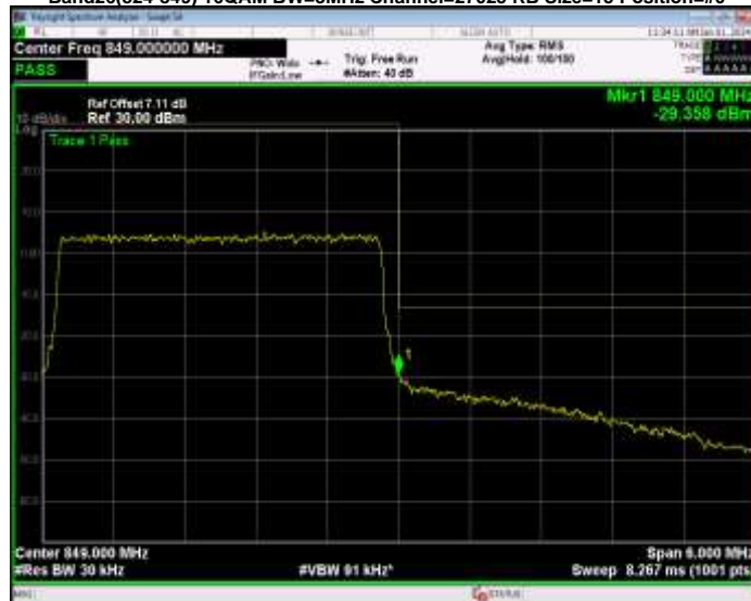
Band26(824-849) 16QAM BW=3MHz Channel=27025 RB Size=15 Position=#0
