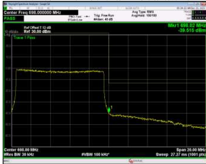
Band71 16QAM BW=15MHz Channel=133197 RB Size=75 Position=#0
