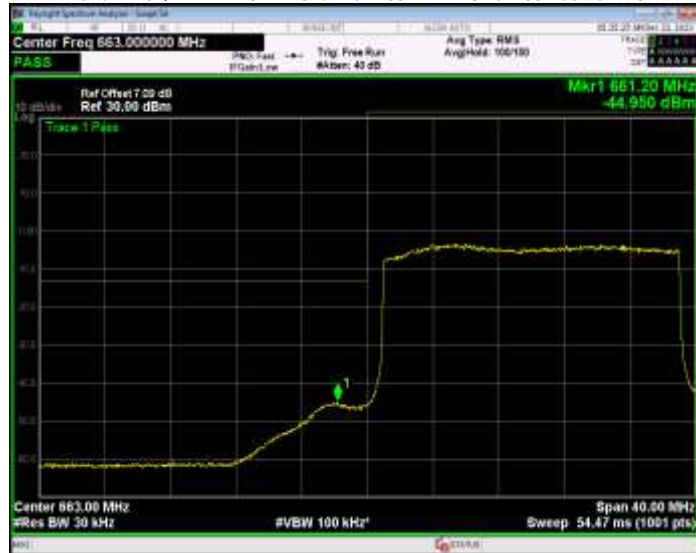
Band71 16QAM BW=20MHz Channel=133372 RB Size=100 Position=#0
