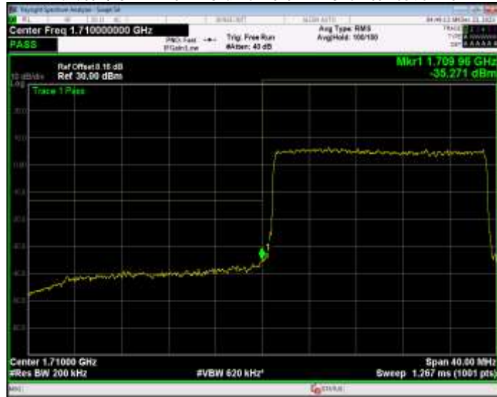
Band66 QPSK BW=20MHz Channel=132572 RB Size=100 Position=#0
