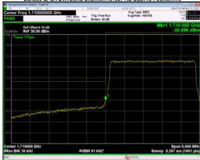
Band66 QPSK BW=3MHz Channel=131987 RB Size=15 Position=#0
