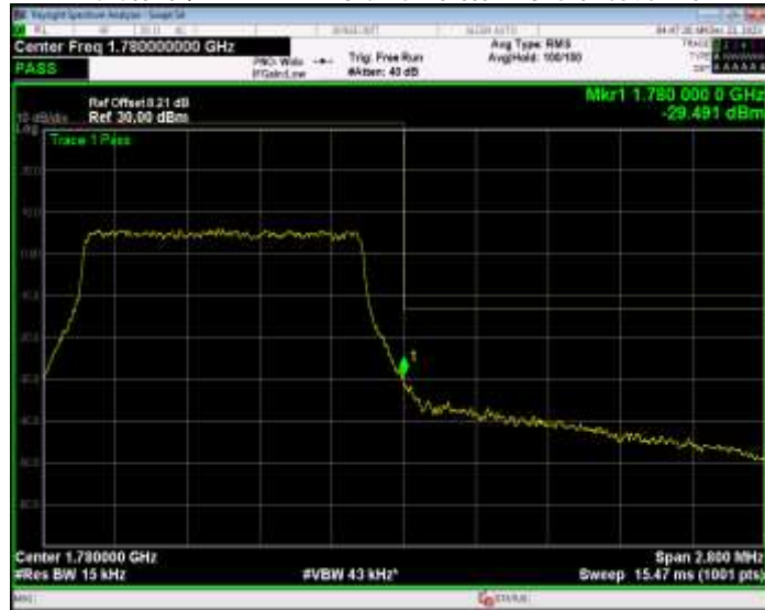
Band66 16QAM BW=10MHz Channel=132022 RB Size=50 Position=#0
