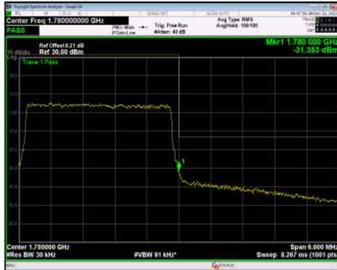
Band66 16QAM BW=5MHz Channel=131997 RB Size=25 Position=#0
