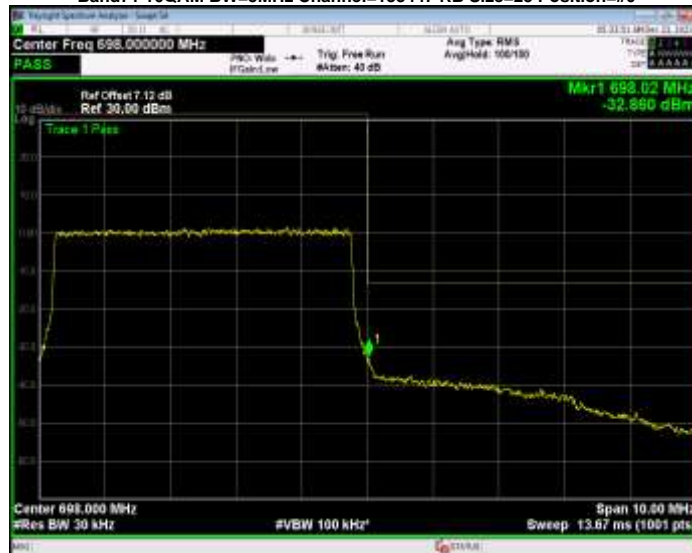
Band71 QPSK BW=10MHz Channel=133172 RB Size=50 Position=#0
