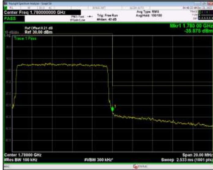
Band66 QPSK BW=15MHz Channel=132047 RB Size=75 Position=#0
