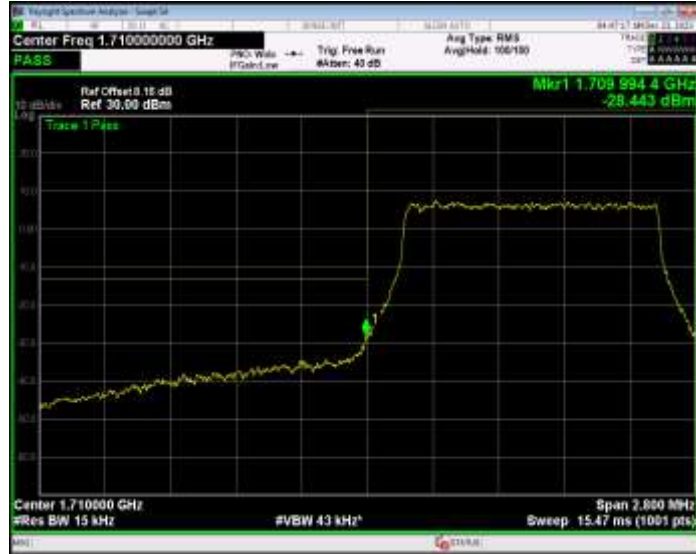
Band66 QPSK BW=1.4MHz Channel=132665 RB Size=6 Position=#0
