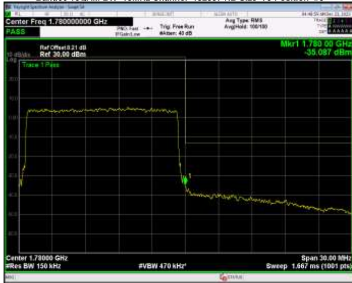
Band66 16QAM BW=15MHz Channel=132597 RB Size=75 Position=#0
