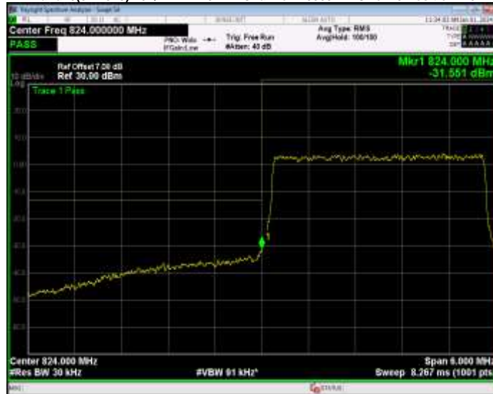
Band26(824-849) 16QAM BW=3MHz Channel=27025 RB Size=15 Position=#0
