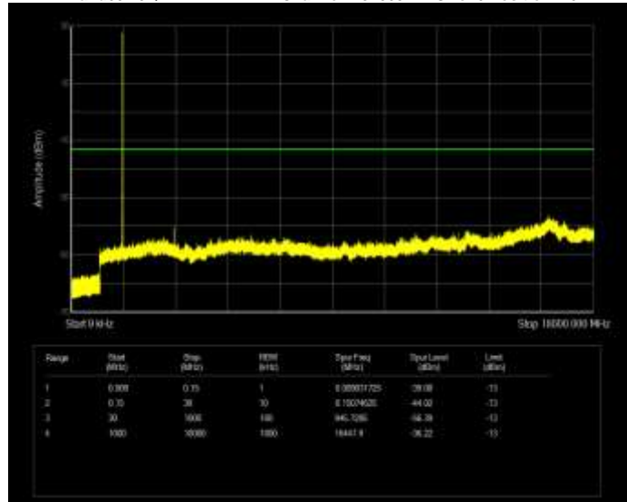
Band66 16QAM BW=10MHz Channel=132022 RB Size=50 Position=#0
