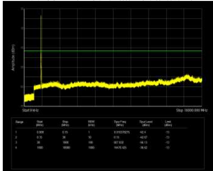
Band4 QPSK BW=10MHz Channel=20175 RB Size=50 Position=#0
