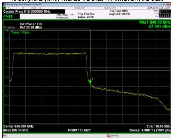
Band26(824-849) QPSK BW=5MHz Channel=27015 RB Size=25 Position=#0
