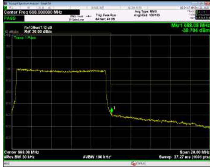
Band71 QPSK BW=15MHz Channel=133197 RB Size=75 Position=#0
