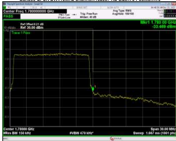
Band66 QPSK BW=15MHz Channel=132597 RB Size=75 Position=#0
