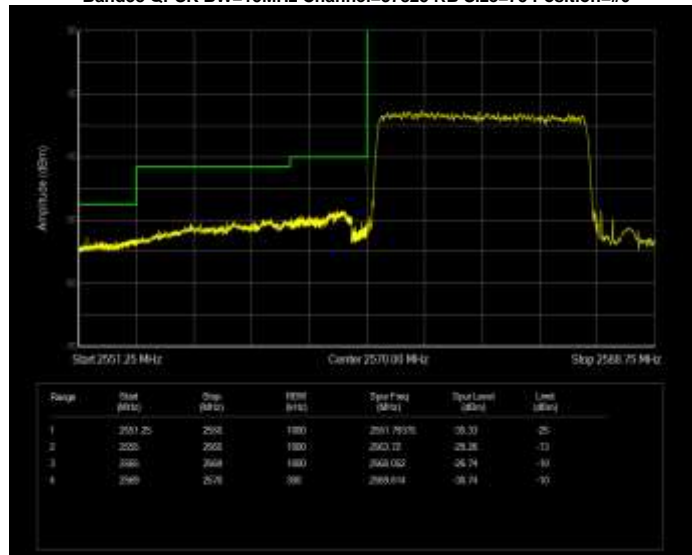
Band38 QPSK BW=15MHz Channel=38175 RB Size=75 Position=#0
