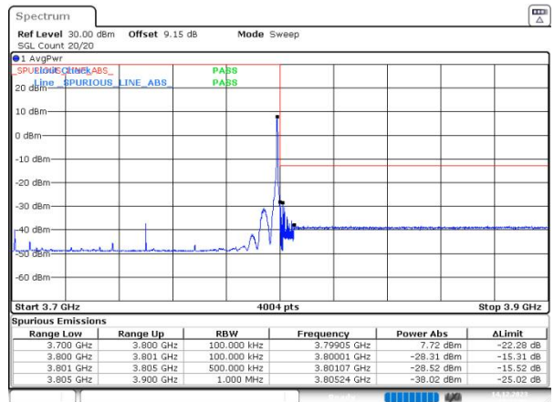
n78(3700-3800) SCS=30kHz DFT_16QAM BW=100MHz HighChannel=650000 RB=1@272
