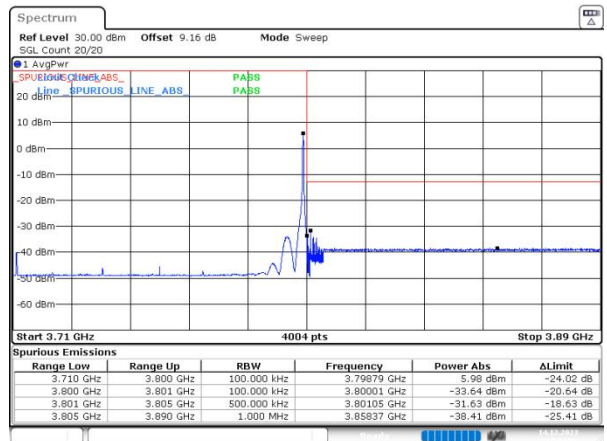
n78(3700-3800) SCS=30kHz DFT_64QAM BW=90MHz HighChannel=650332 RB=1@244
