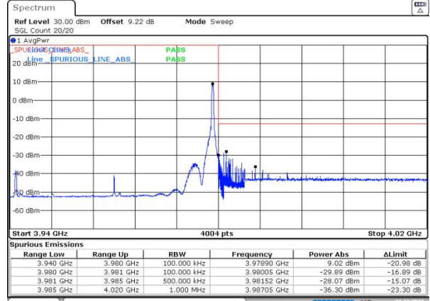
n77(3700-3980) SCS=30kHz DFT_256QAM BW=40MHz HighChannel=664000 RB=1@105
