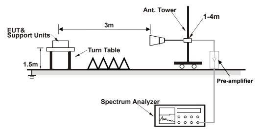
For radiated test above 18GHz
