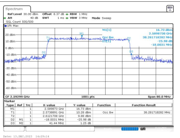
n41 SCS=30kHz CP_64QAM BW=40MHz Channel=518598 RB=106@0
