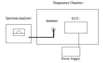
The EUT which is powered by the Battery, is coupled to the Spectrum Analyzer; the RF load attached to the EUT antenna terminal is 500hm; the path loss as the factor is calibrated to correct the reading 5.4 EUT OPERATION CONDITIONS
