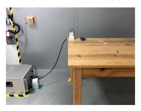
Set-up for Radiated Emission (RE), Below 1GHz
