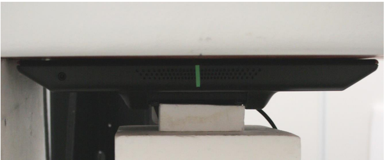
Front side of the device against the phantom, 0 mm separation distance
