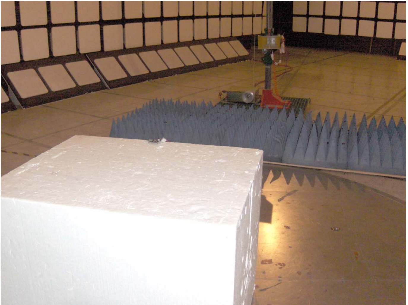
Transmitter Radiated Emissions at 3 m Distance Orthogonal Position 1
