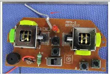
The antenna is integrated on the main PCB and no consideration of replacement. The best case gain of the antenna is 0.8dBi.
