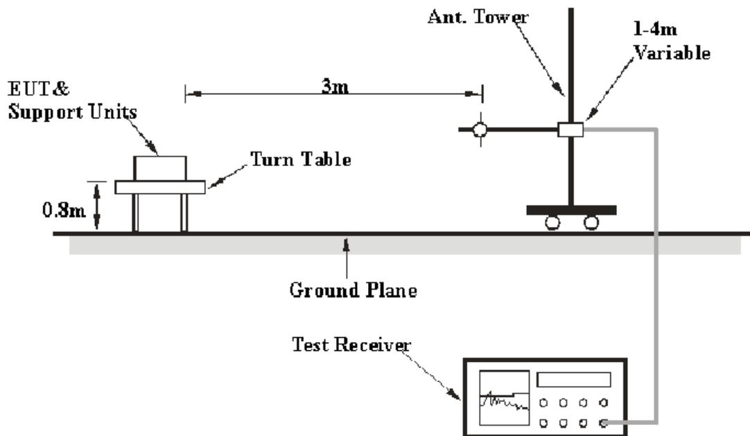
The radiated emission tests were performed in the 3 meters chamber test site, using the setup accordance with the ANSI C63.4-2009. The specification used was the FCC 15.209, and FCC 15.247 limits.
