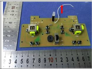
The antenna is integrated on the main PCB and no consideration of replacement. The best case gain of the antenna is 1.3dBi.
