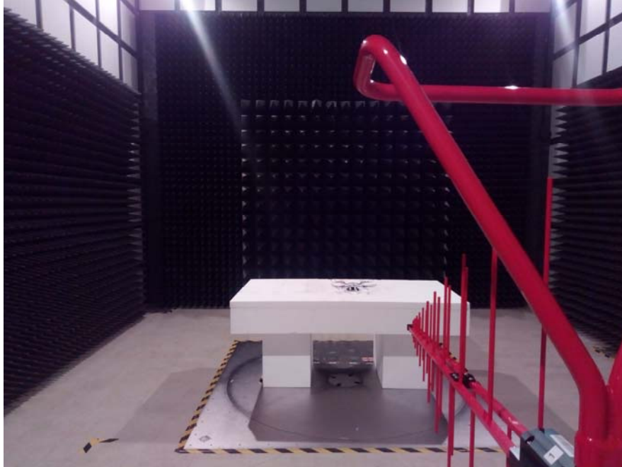
Radiated Emissions View (Below 1 GHz)
