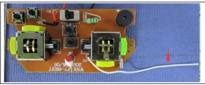
The antenna is integrated on the main PCB and no consideration of replacement. The best case gain of the antenna is 1.3dBi.
