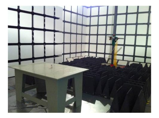
**Radiated Emissions Test Setup**
