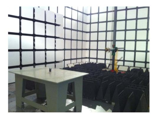
**Radiated Emissions Test Setup**
