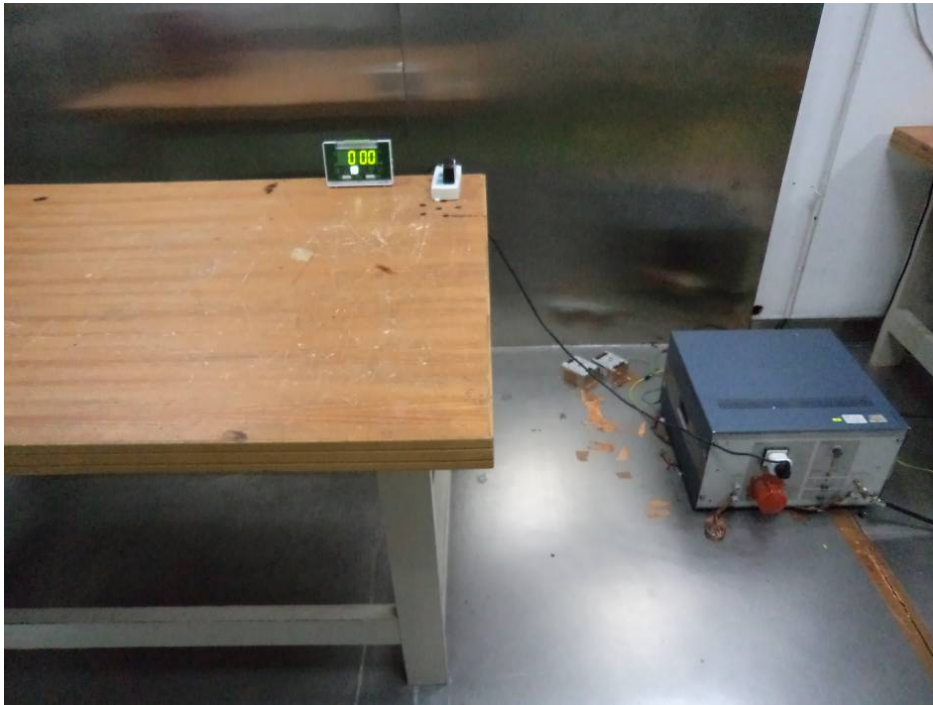
Conducted Emissions - Rear View
