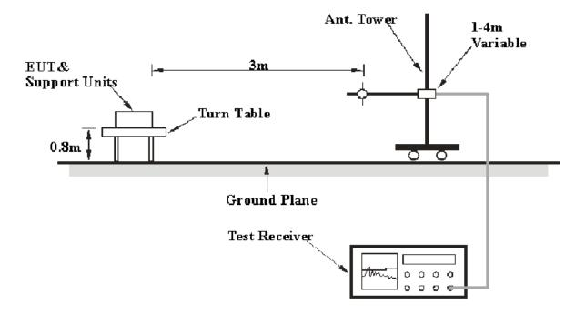
The radiated emission and out of band emission tests were performed in the 3 meters, using the setup accordance with the ANSI C63.4-2009. The specification used was the FCC 15.209 and FCC 15.249 limits.
