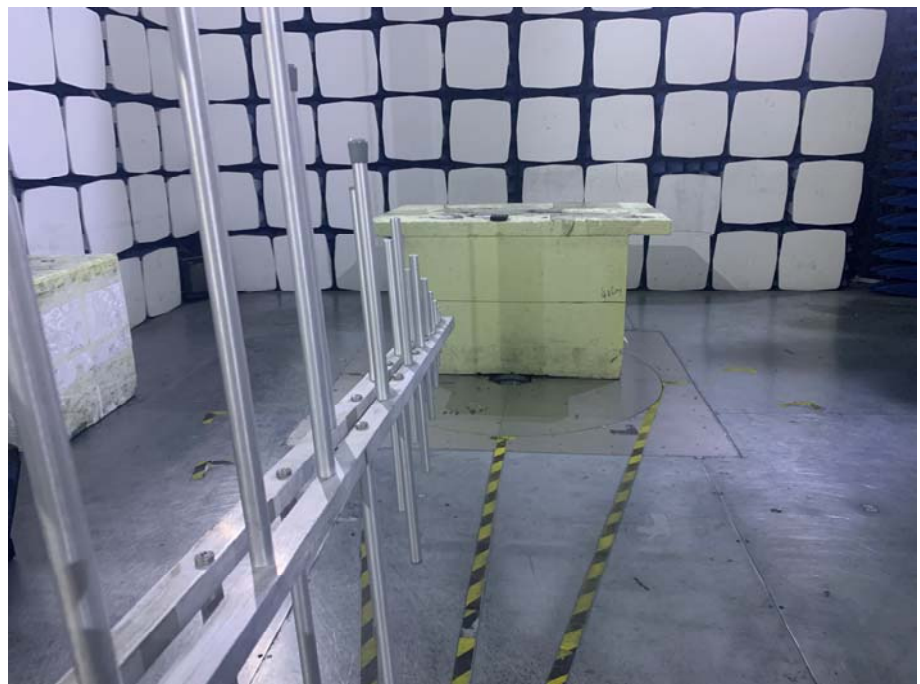
Radiation Emission Test Setup (30MHz to 1GHz)
