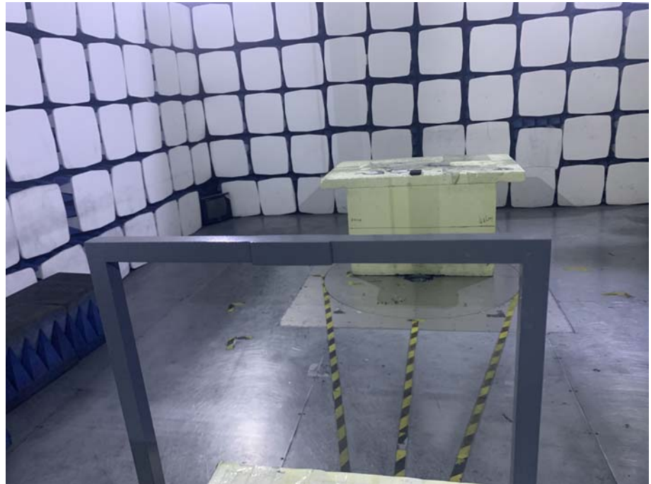
Radiation Emission Test Setup (Below 30MHz)
